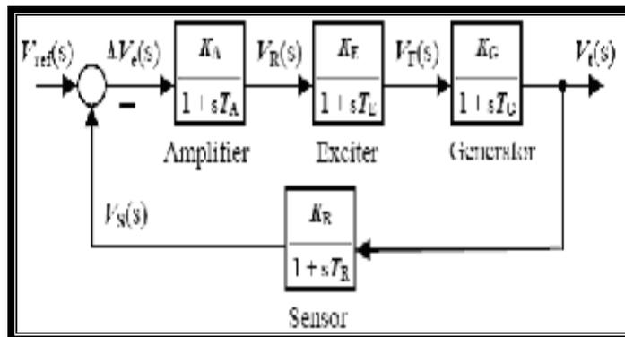
Figure (4) Block diagram of a simple AVR [11]
