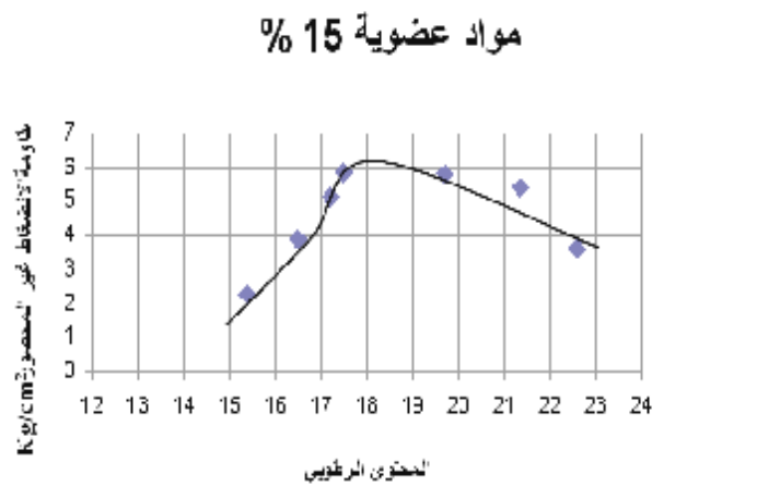
Figure (5-d) Modified Compaction Curve with unconfined compression strength
