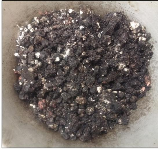
Figure 5. Asphalt specimen with C&DWMs after mixing and compaction.
