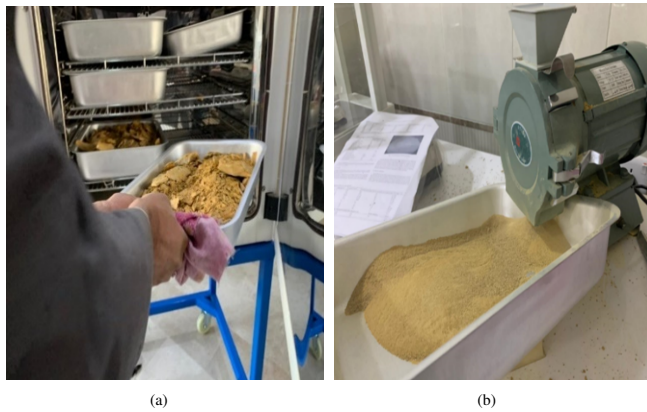
Figure 1. The preparation process of bentonite, (a) the Drying process, and (b) the Grinding process.
