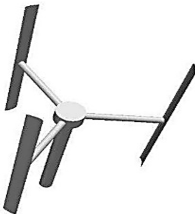
Figure 1. H-type vertical axis wind turbine [41].
