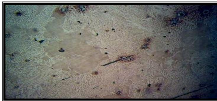
Figure (11): Microstructure Alloy Steel specimen forged with load 800 ton. [X 300] the structure is matrix of three phase  $\{((\text{FeCr})_7\text{C}_3), \text{Bainite}, \text{and Martensite}\}$  L Grain size = 66mm S Grain size = 3mm
