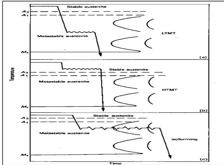
Figure (1): Schematic diagrams of thermochemical treatment<sup>[6]</sup>:
