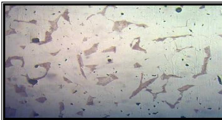
Figure (13): Microstructure Alloy Steel specimen forged with load of 2500 ton [X 300], three phases{( Fe-Cr), Bianite, (FeCr)<sub>7</sub>C<sub>3</sub>}, Grain size = 20.2 mm
