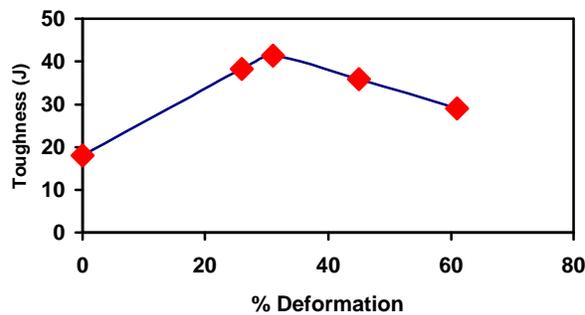
Figure (8) :Effect of deformation percentage on the toughness.
