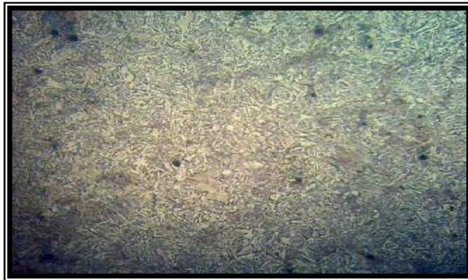
Figure (10): Microstructure of Alloy Steel specimen Before T.M.T. [X 300], two phases  $\{(\alpha\text{-Fe}), (p, (\alpha+\text{Fe}_3\text{C}))\}$  Grain size = 5 mm
