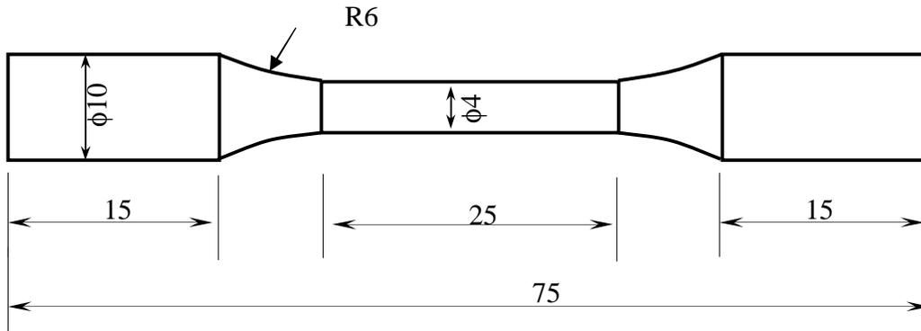
Figure (6): Tensile specimen (all Dim. in mm).
