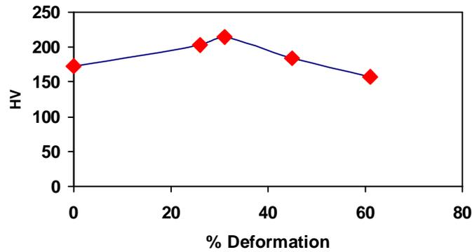
Figure (9): Effect of deformation percentage on the hardness.
