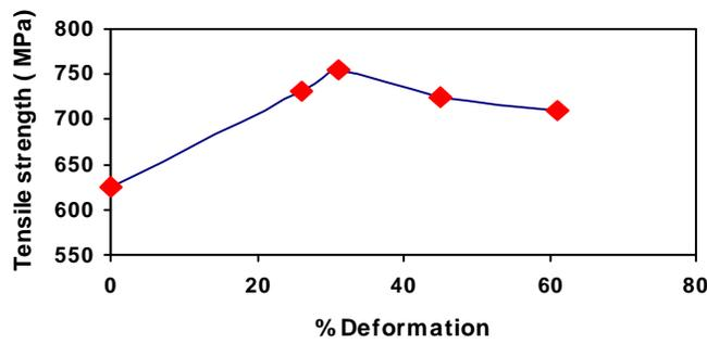
Figure (7) Effect of deformation percentage on the tensile strength.
