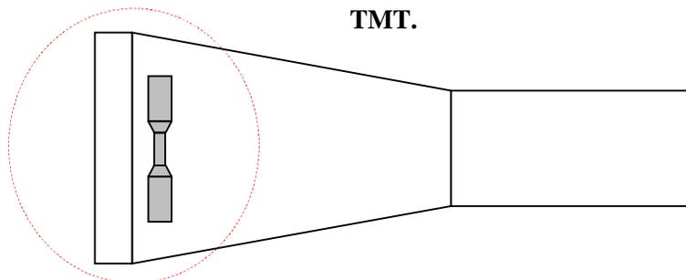
Figure (5): Location of the sampled tensile specimen
