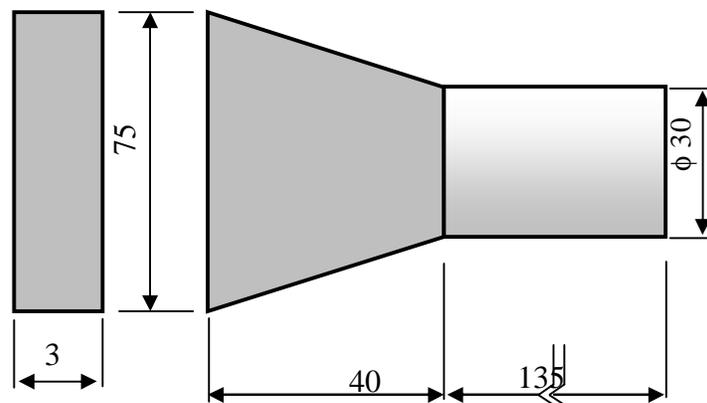
Figure (4): Specimen (1) Dimensions after TMT.
