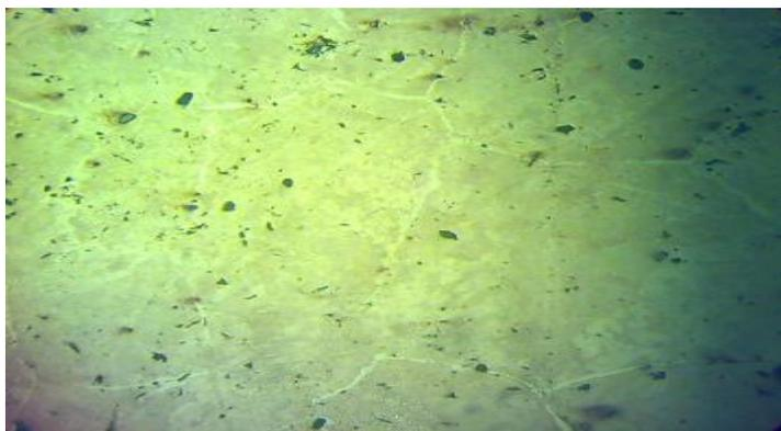
Figure (14): Microstructure AlloySteel specimen forged with load of 4000 ton. [X 300] , two phases { perlite,(a+Fe<sub>3</sub>C) , (FeCr) }. Grain size = 71.4 mm
