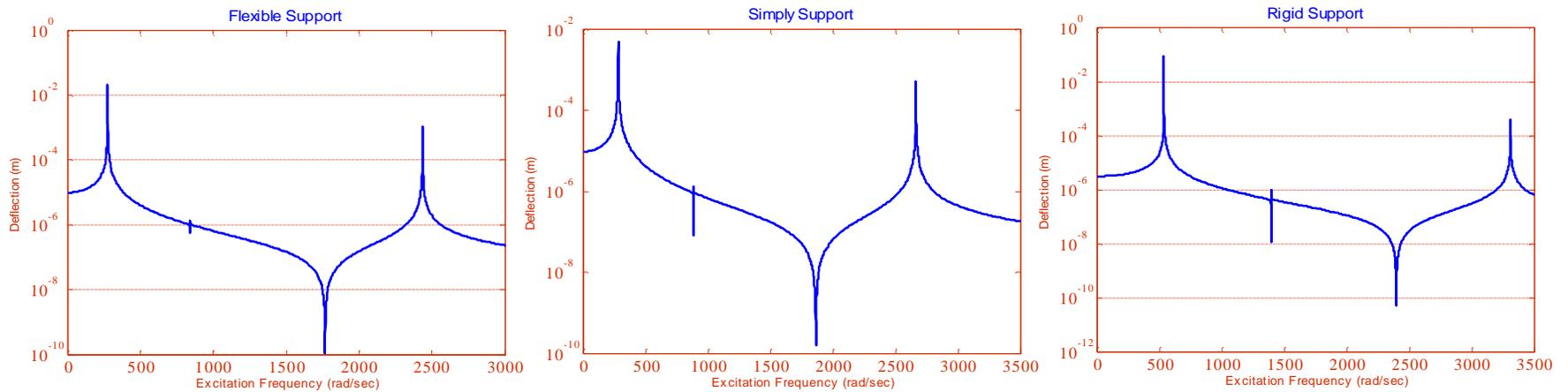
Figure (6) Deflection for (flexible, simply, rigid) supports pipe without fluid with various excitation frequencies at mid span of aluminum pipe (model-1) represent three lowest natural frequency.
