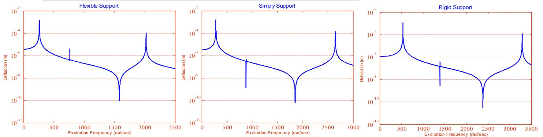
Figure (5) Deflection for (flexible, simply, rigid) supports pipe without fluid with various excitation frequencies at mid span of steel pipe (model-1) represent three lowest natural frequency.
