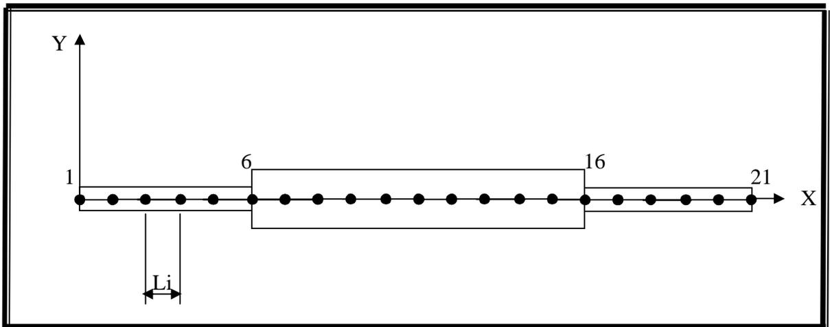
Figure (2) Pipe with discrete elements and masses.
