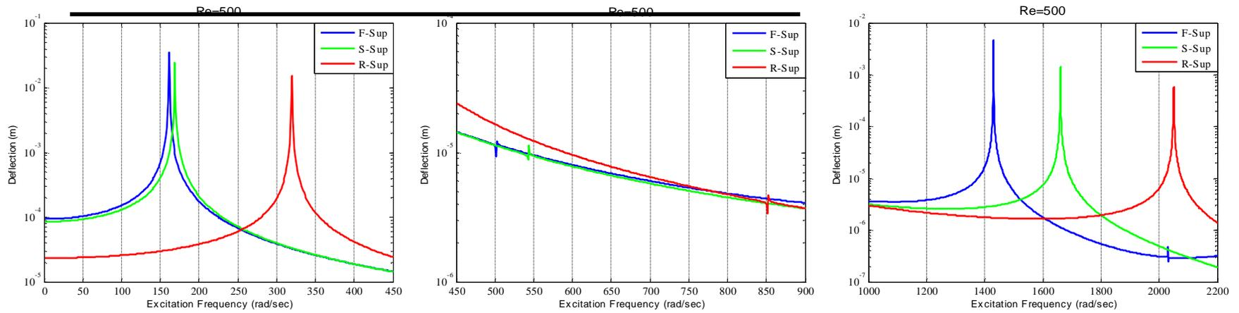
Figure (8) Deflection for (flexible, simply, rigid) supports pipe conveying fluid with various excitation frequencies at mid span of copper pipe (model-1) represent (1<sup>st</sup>, 2<sup>nd</sup>, 3<sup>rd</sup>) natural frequency for Re=500.
