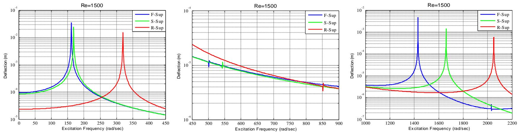
Figure (9) Deflection for (flexible, simply, rigid) supports pipe conveying fluid with various excitation frequencies at mid span of copper pipe (model-1) represent (1<sup>st</sup>, 2<sup>nd</sup>, 3<sup>rd</sup>) natural frequency for Re=1500.
