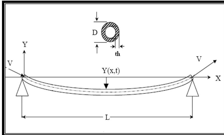
Figure (1) Pipe conveying fluid.
