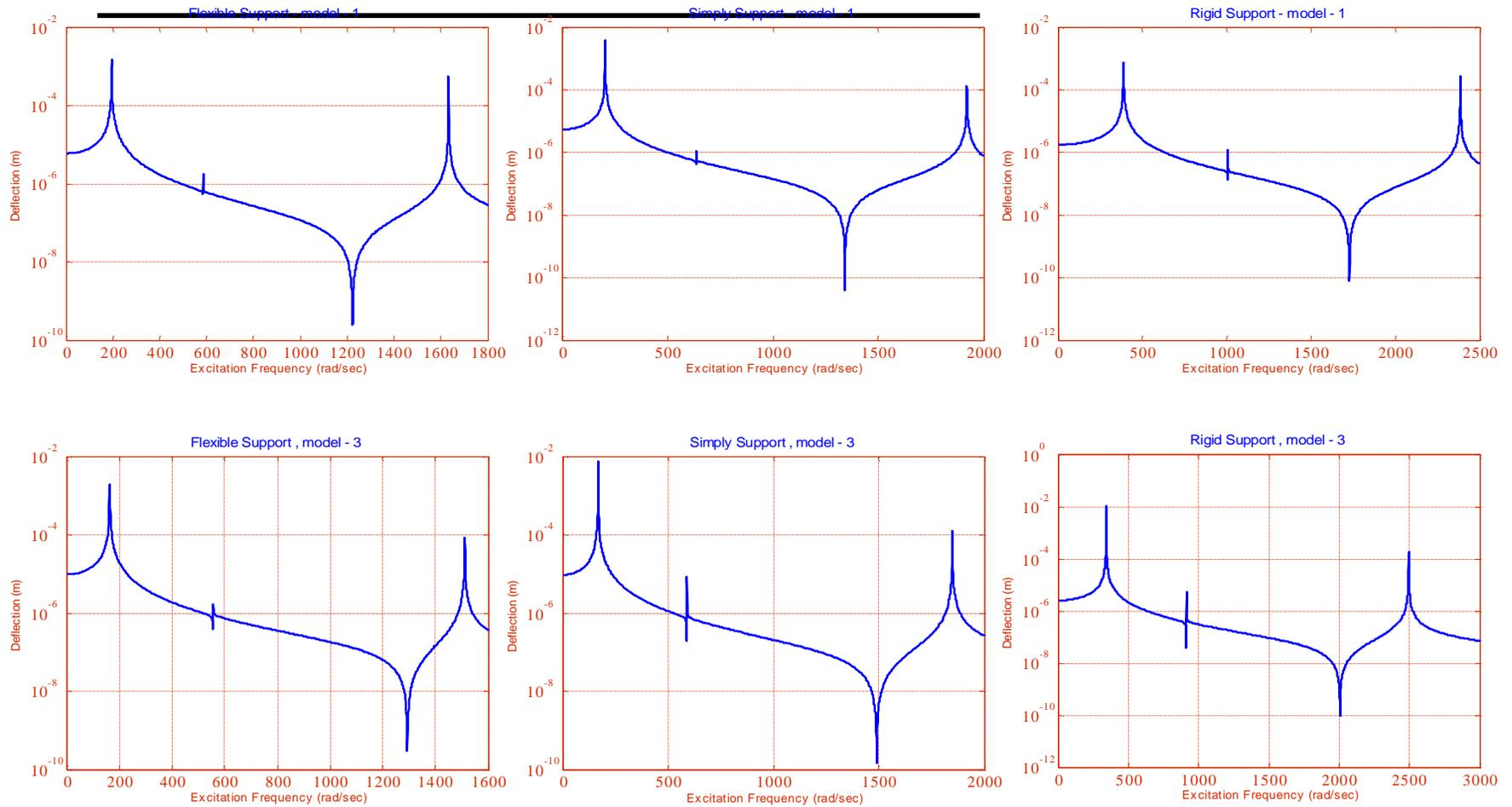
Figure (7) Deflection for (flexible, simply, rigid) supports pipe without fluid with various excitation frequencies at mspan of copper pipe with different lengths (model-1, model-3) represent three lowest natural frequency.
