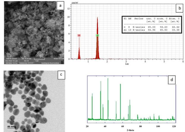
Figure 2. The characterization of nano-Al<sub>2</sub>O<sub>3</sub> particles (a) SEM, (b) EDAX elemental composition and (c) TEM and (d) XRD.
