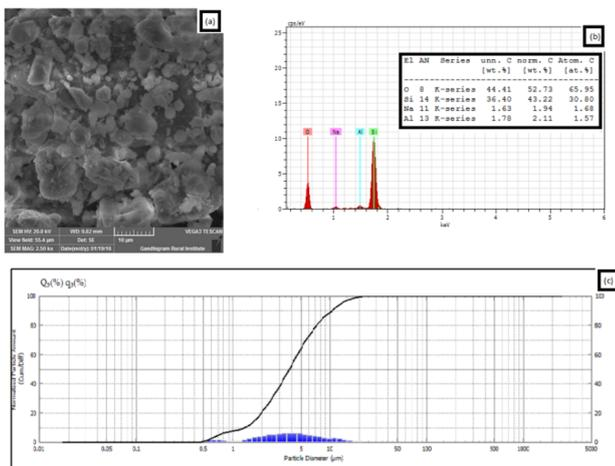
Figure 1. The characterization silica fume.
