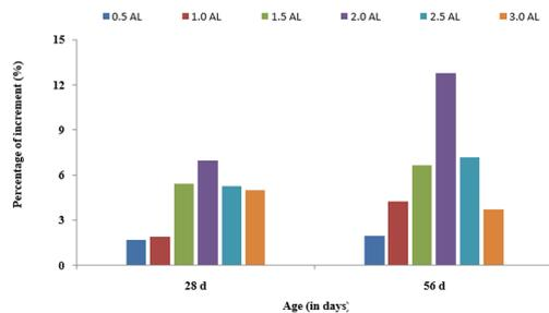
Figure 5. The percentage of enhancement in modulus of elasticity.
