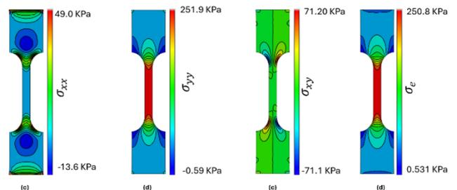
Figure 12. Typical full-field stress of the rubber specimen with zero epoxy ratio subjected to uniaxial extension. Where: a) The transverse stress  $\sigma_x$ ; b) The longitudinal stress  $\sigma_y$ ; c) The shear stress  $\sigma_{xy}$ ; and d) The Von-mises stress, equivalent stress  $\sigma_e$ .
