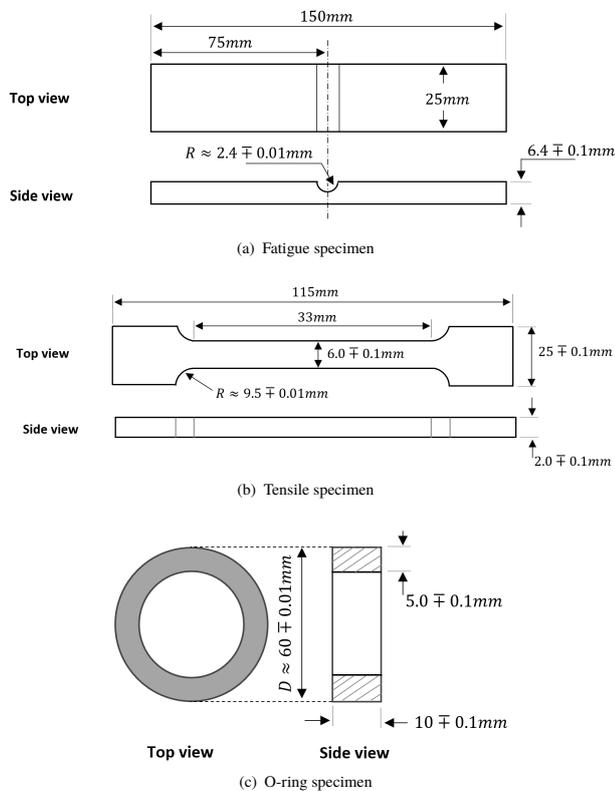
**Figure 2.** Schematic of the specimens used in this test where (a) The fatigue test specimen, (b) The tensile test specimen, and (c) the O-ring modulus specimen.
