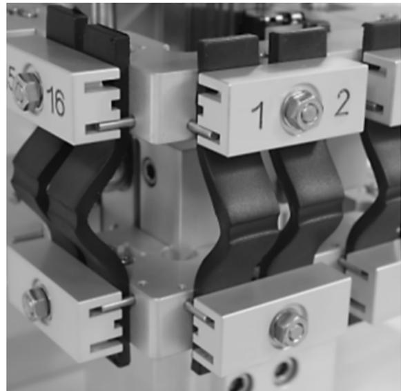
**Figure 3.** Fatigue testing device (De Mattia Flexing Machine).
