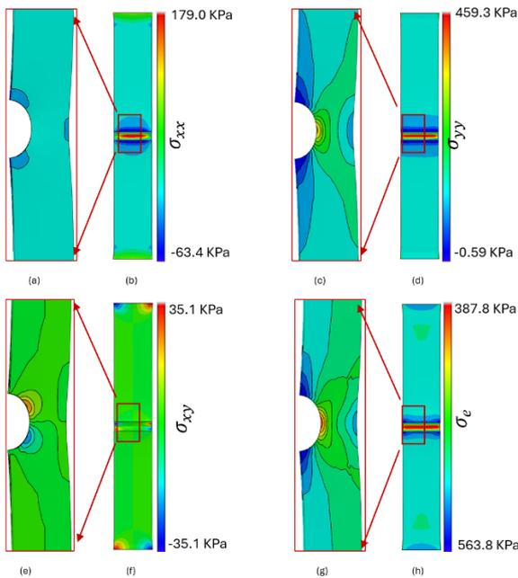
**Figure 13.** Typical Full-field stress of the rubber fatigue specimen with zero epoxy ratio subjected to uniaxial extension. Where: a, b) The transverse stress  $\sigma_{xx}$ ; c, d) The longitudinal stress  $\sigma_{yy}$ ; e, f) The shear stress  $\sigma_{xy}$ ; and g, h) The Von-mises stress, equivalent stress.
