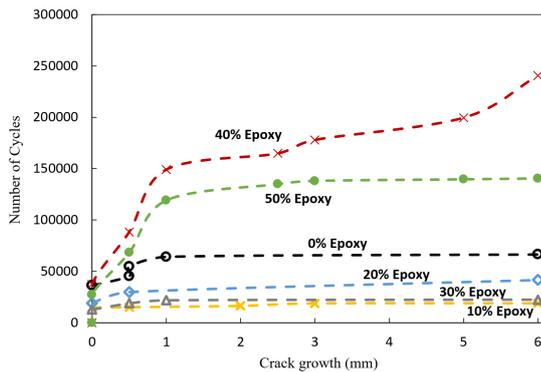
Figure 9. The fatigue life and crack growth of the specimen subjected to tensile periodic load
