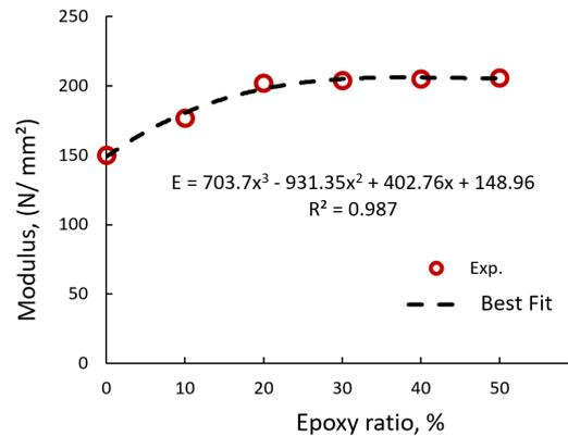
Figure 10. The typical relationship between the modulus of rubber epoxy specimens vs epoxy ratio.
