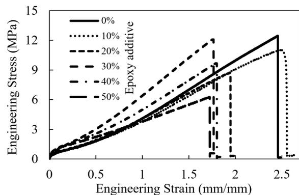
**Figure 6.** Typical experimental results of the stress-strain of the rubber epoxy with different additive amounts according to the ASTM D412.
