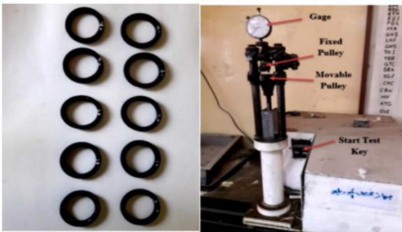
**Figure 4.** Specimens' preparation and testing machine (a) Modulus test samples, (b) Modulus test device.
