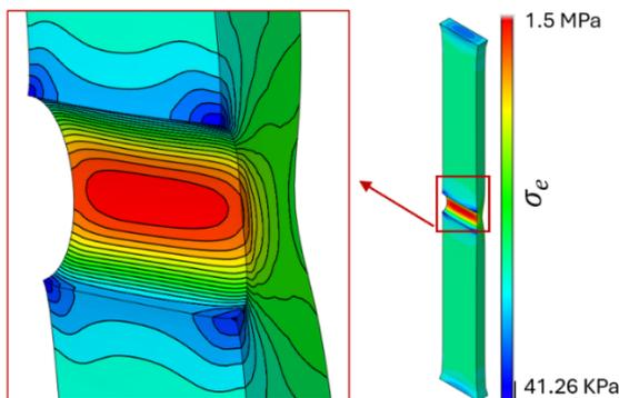
**Figure 14.** Typical Von-mises stress distribution of fatigue specimen subjected to 10mm displacement along the longitudinal direction
