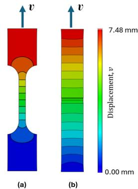
Figure 11. A typical displacement profile of testing rubber with zero epoxy ratio, where a) Tensile specimen, b) Fatigue specimen.
