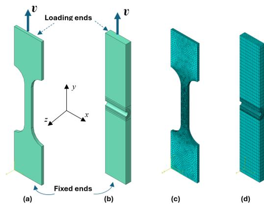
**Figure 5.** The CAD and FE model of the Tensile and fatigue specimens. Where a) the dog-bone tensile specimen, b) the rectangular with semicircle groove specimens, c, and d) the mesh model of the tensile and fatigue specimens respectively.
