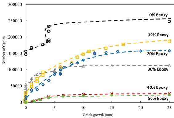
Figure 8. The fatigue life and the length of the crack under the bending test
