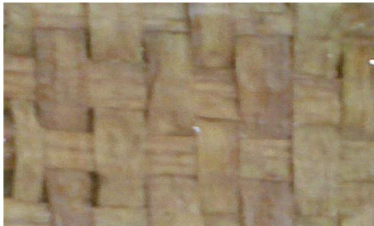
**Figure (1) pseudo-stem banana fibers in the woven fabric configuration**
