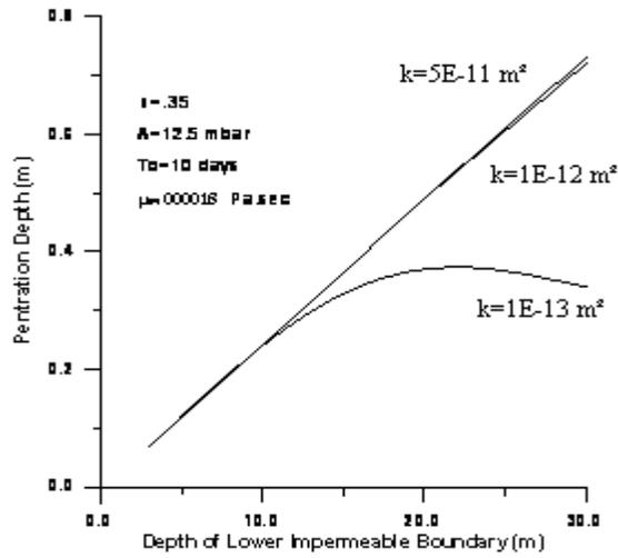
Figure (4) Penetration Depth or Different Soil Settings
