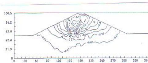
Fig. (20) Ver. Disp. Contours, Const. w.c=19.5 / W.L at Elev. 115 (-ve disp).
