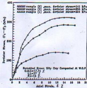
Fig. (5-a) Consolidated Undrained Triaxial Test With P.W.P. Measurements, Quarry No. (4).
