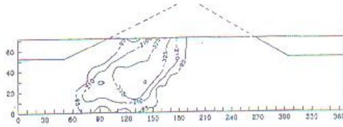
Fig. (15) PWP Contours, Const. w.c=20.5 / 2nd H.U. (- comp).
