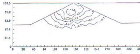
Fig. (21) Ver. Disp. Contours, Const. w.c=20.5 / W.L at Elev. 115 (-ve disp).
