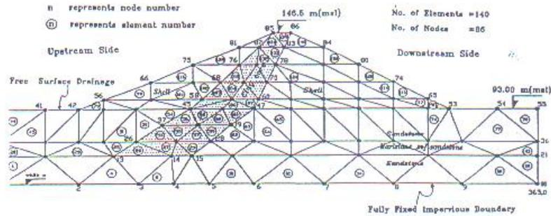
Fig. (11) Finit Element Mesh Used to Analyze The Great Earth Dam,
