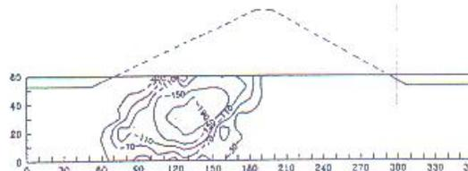
Fig. (14) PWP Contours, Const.  $w_c = 29.5 / 1st \text{ lift} (- \text{ comp.})$ .
