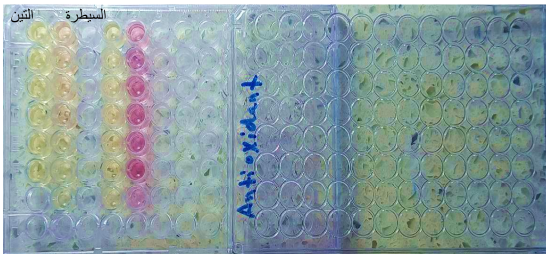
Figure (4): MTP 96-well precision titration plate for antioxidant activity testing to measure the absorbance of the sample As and the absorbance of the control Ac.
