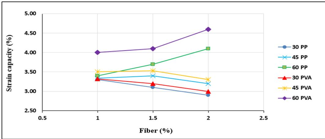
**Figure 4:** Strain capacity with different fiber contents and types
