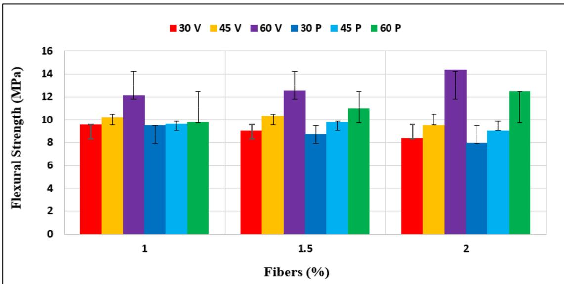
Figure 3: Error bars of Standard deviation of flexural strength for different fiber contents in bendable concrete mixes
