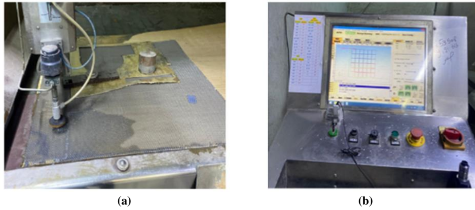
Figure 4: Water jet cutters (a) nozzle (b) computer
