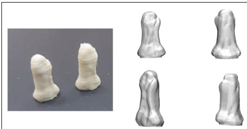
**Figure 9:** The Second Virtual Model of a 3D-printed Finger Distal Phalanx after Processing the Holes
