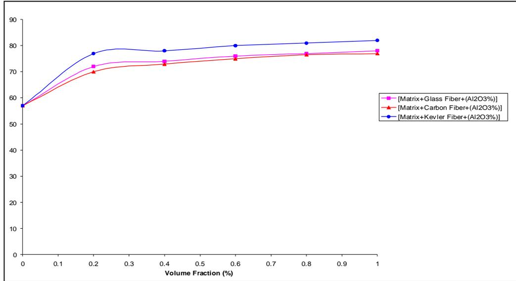
Figure (5): Effect of additive Al<sub>2</sub>O<sub>3</sub> on hardness test of polyester composite system.
