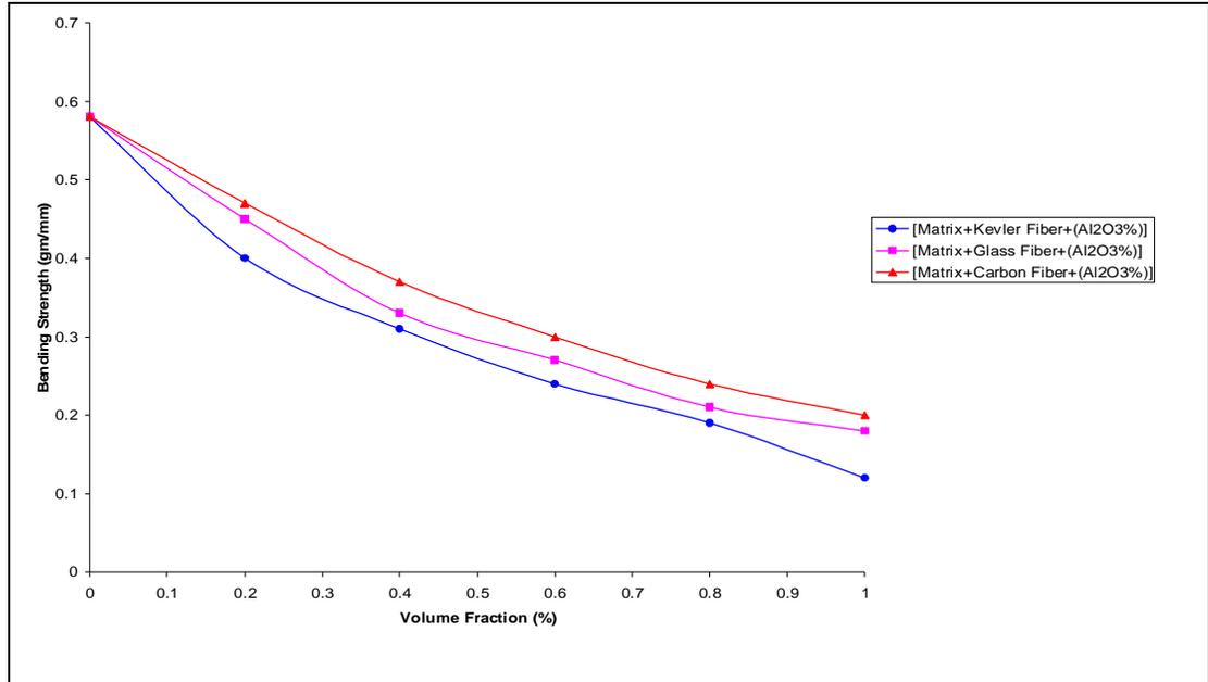
Figure (1): Effect of additive Al<sub>2</sub>O<sub>3</sub> on bending strength of polyester composite system.
