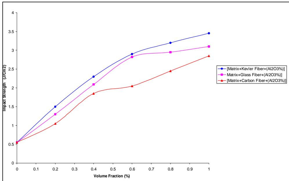
Figure (4): Effect of additive Al<sub>2</sub>O<sub>3</sub> on impact strength of polyester composite system.
