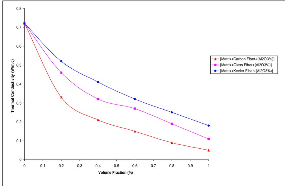
Figure (7):Effect of additive Al<sub>2</sub>O<sub>3</sub> on thermal conductivity of polyester composite system.
