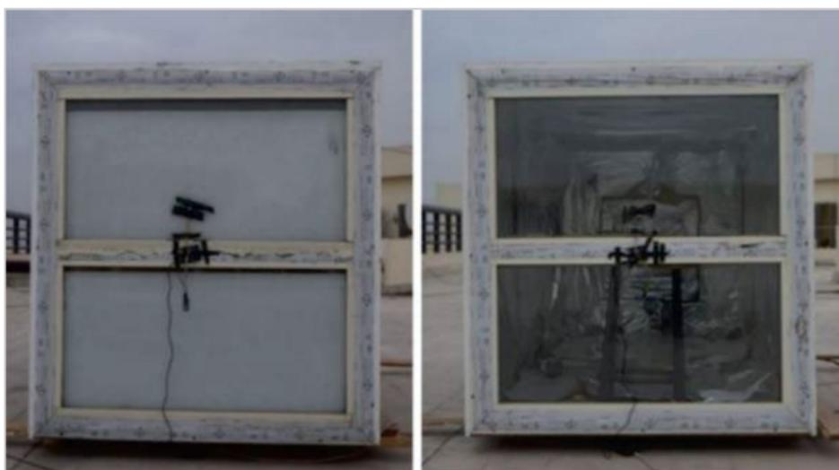
Figure 3: Experimental Setup (A) Façade Filled with PCM (B) Façade Filled with Air [22]
