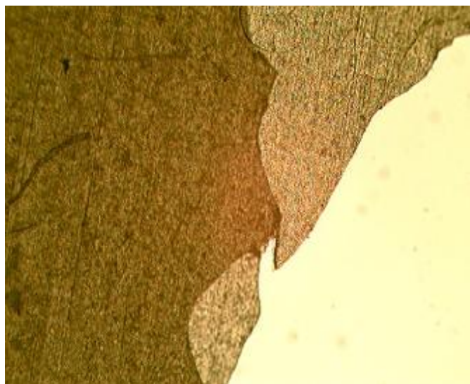
Figure (7) Optical microscope image of the two distinct sheets of aluminum with measured thicknesses approximately 10 μm (each).
