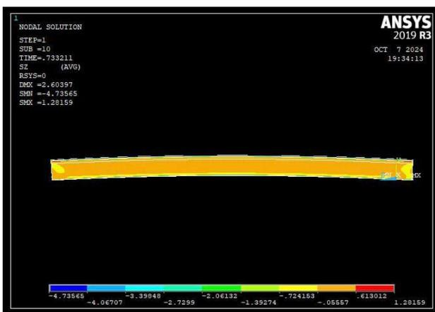
Fig. 13 The Von Mises Stress for Girder 3.
