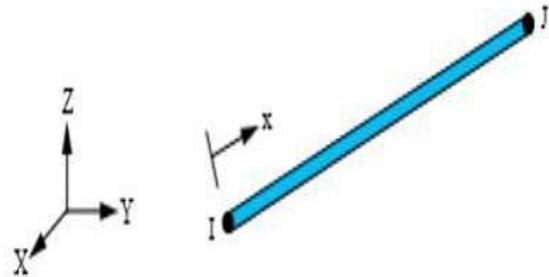
**Fig. 2** Beam188 Element (ANSYS Help) [9].
