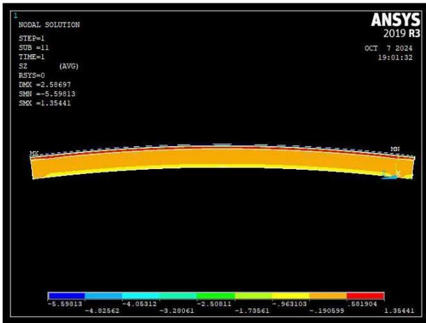
Fig. 11 The Von Mises Stress for Girder1
