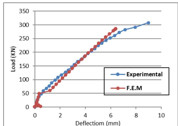
**Fig. 5** Load Deflection curves for Experimental and Numerical results.
