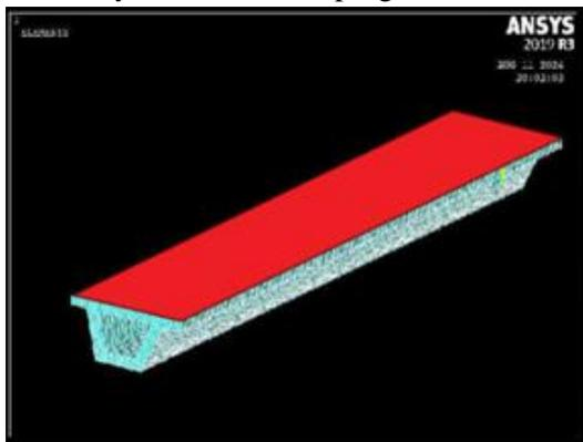
a) Girder1(Thermal load at Upper Flange)
