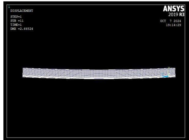
**Fig. 9** The deflected shape for Girder2.
