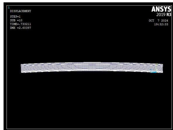
**Fig. 10** The deflected shape for Girder3.
