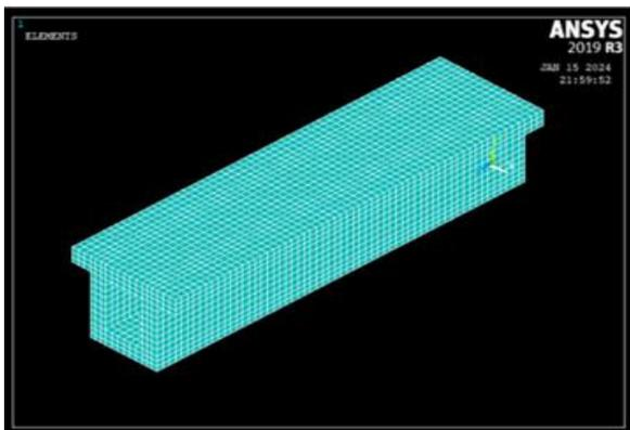
**Fig. 4** Finite element meshing of RC box girder
