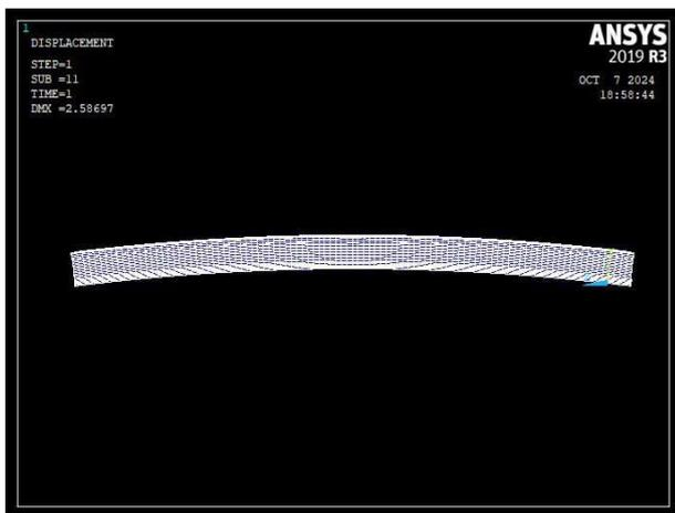
**Fig. 8** The deflected shape for Girder1
