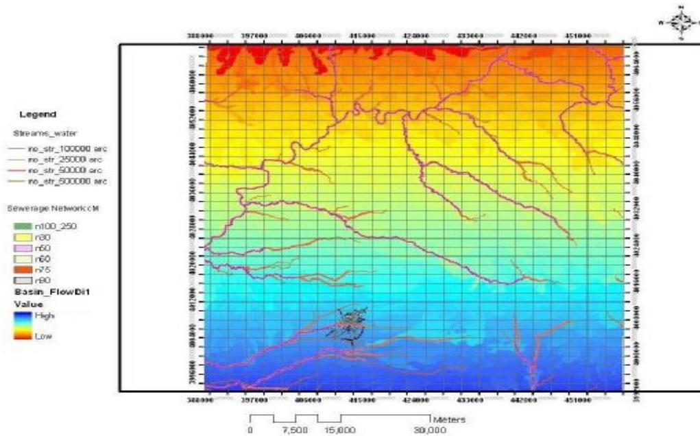
Figure (3b) Flow Model of water illustrates surface water & the basin (The more saturated areas) over an elevation surface
