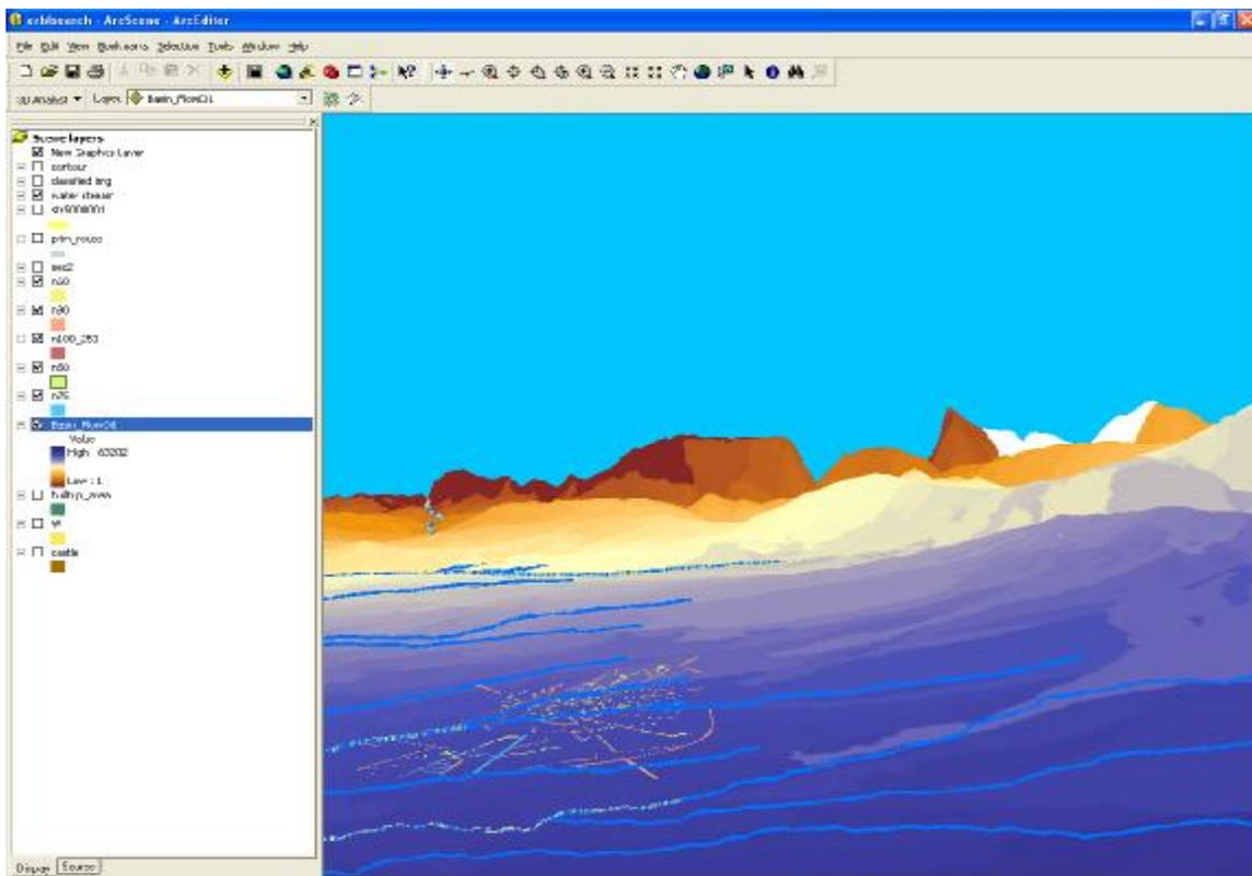
Figure (4d) A Flow basin of Erbil City has been draped over the terrain DEM
