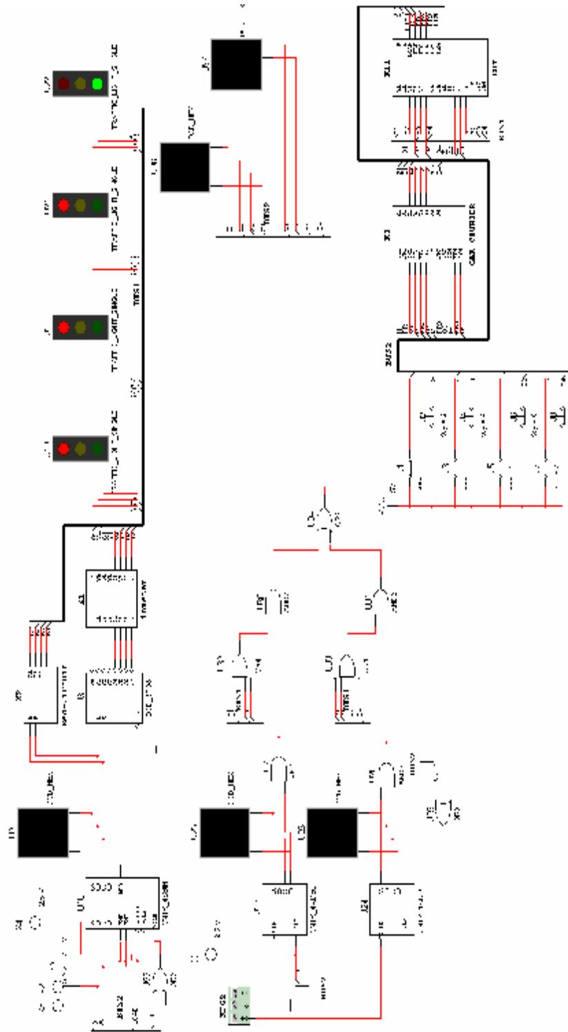
Figure (2): The Proposed Design of Intelligent Traffic Light System.
