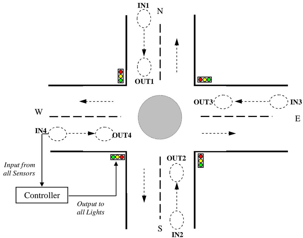
Figure (1): Schematic view of road intersection and traffic light system
