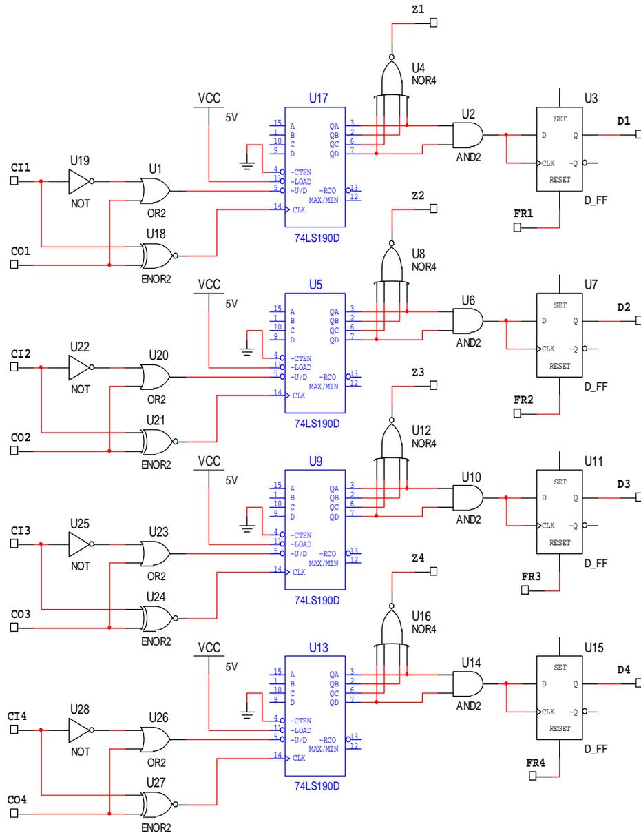
Figure (3): CAR COUNTER Circuit.
