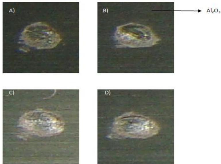
Figure (A3) Optical Images magnified (1x20) after Irradiated by Nd-YAG Pulsed laser A) 24 volts B) 21 volts C) 19 volts D)15.5 volts (Surface Treated by laser Before Anodizing) Anodizing Time is 30 Minutes, 360mJ energy,  $3 \times 10^{-9}$  pulsed duration
