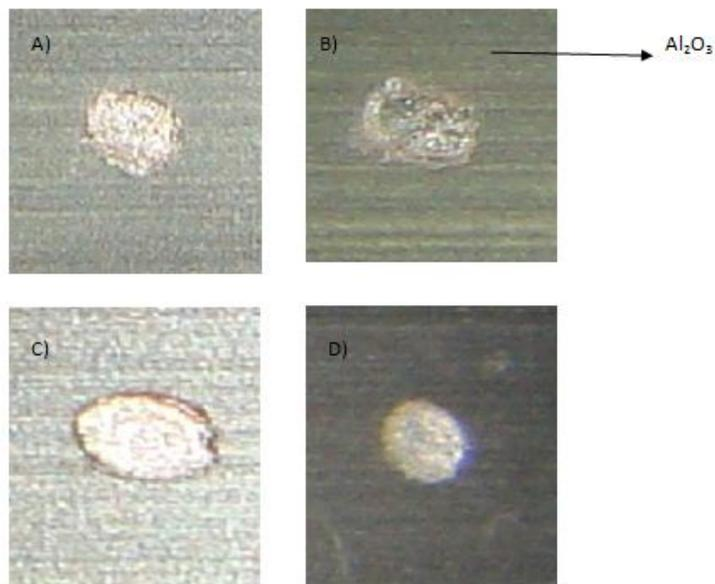
Fig (A4) Optical Images magnified (1x20) after Irradiated by Nd-YAG Pulsed Laser A) 24 volts B) 21 volts C) 19 volts D)15.5 volts (Surface was not Treated by Laser Before Anodizing) Anodizing Time is 30 Minutes, 360mJ energy,  $3 \times 10^{-9}$  pulsed duration
