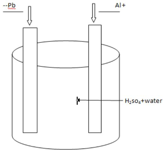
Figure (A1) shows the experimental setup of anodizing
