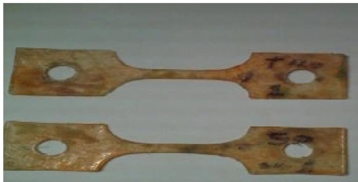
Figure (6) Photograph of composite creep test specimen
