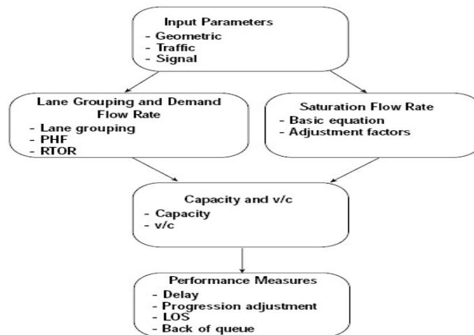
Figure (2) Signalized intersection methodology.
