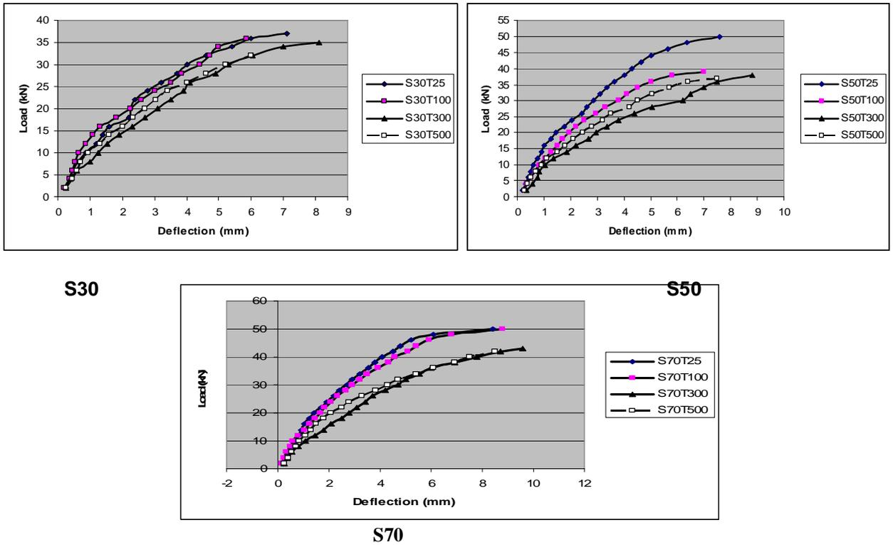
Figure (7): load Deflection Curves for Slabs in Series 1(Square Specimens)
