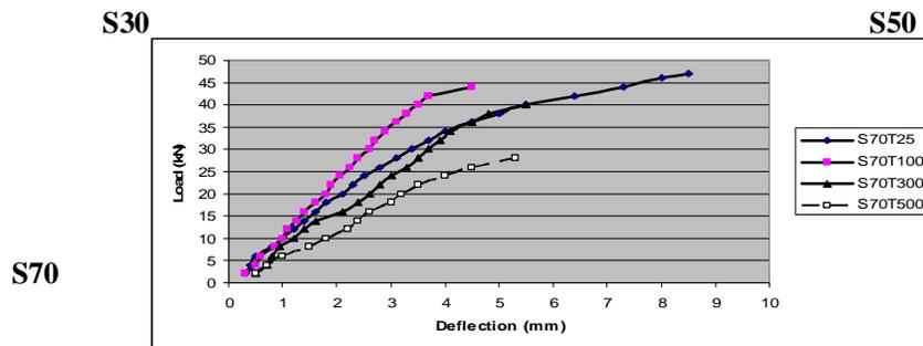
Figure (8): load Deflection Curves for Slabs in Series 2 (Trapezoidal Specimens)
