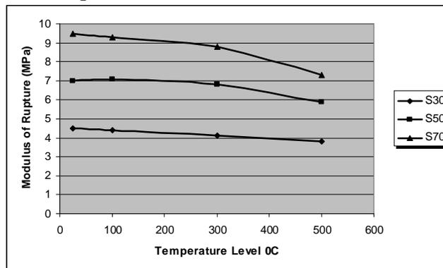
Figure (4): The Relation between Modulus of Rupture and Temperature level for all Mixes
