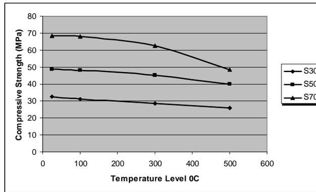
Figure (3): The Relation between Compressive Strength and Temperature level for all Mixes
