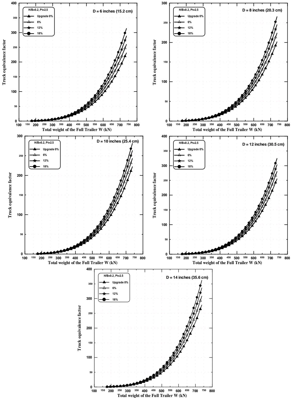
Figure (6) Equivalence factors for Full-Trailers of type 1.2+2.2 on upgrades, for  $H/B=0.2$ ,  $p_t=2.5$ , and  $D=6, 8, 10, 12,$  and  $14$  inches (15.2, 20.3, 25.4, 30.5 and 35.6 cm).
