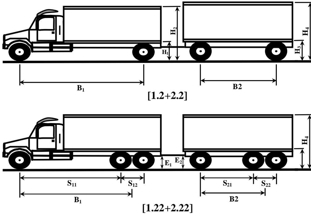
Figure (2) Vehicles dimensions for (1.2+2.2) and (1.22+2.22) full-trailers.
