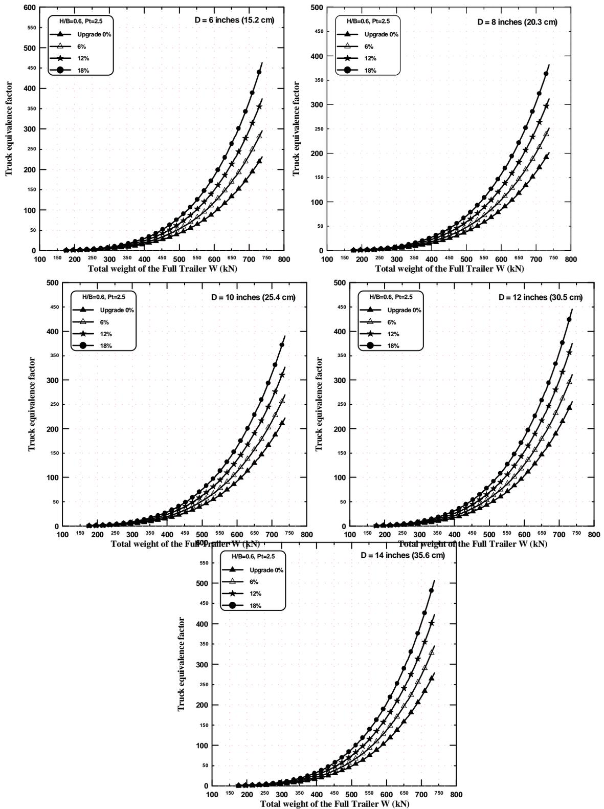
Figure (7) Equivalence factors for Full Trailers of type 1.2+2.2 on upgrades, for  $H/B = 0.6$ ,  $p_t=3$ , and  $D=6, 8, 10, 12,$  and  $14$  inches (15.2, 20.3, 25.4, 30.5 and 35.6 cm).
