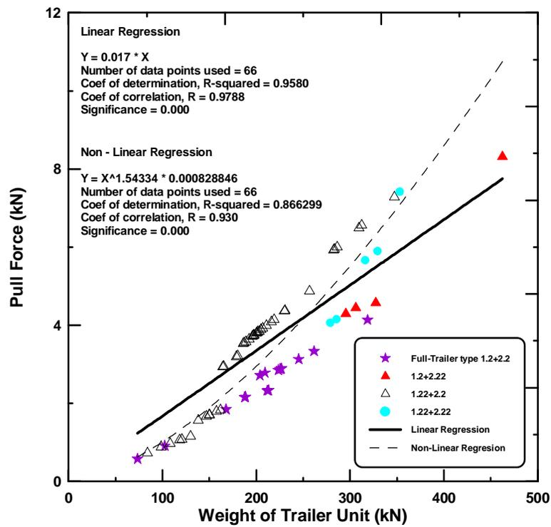
Figure (1) Correlation between pull force and weight of trailer unit.
