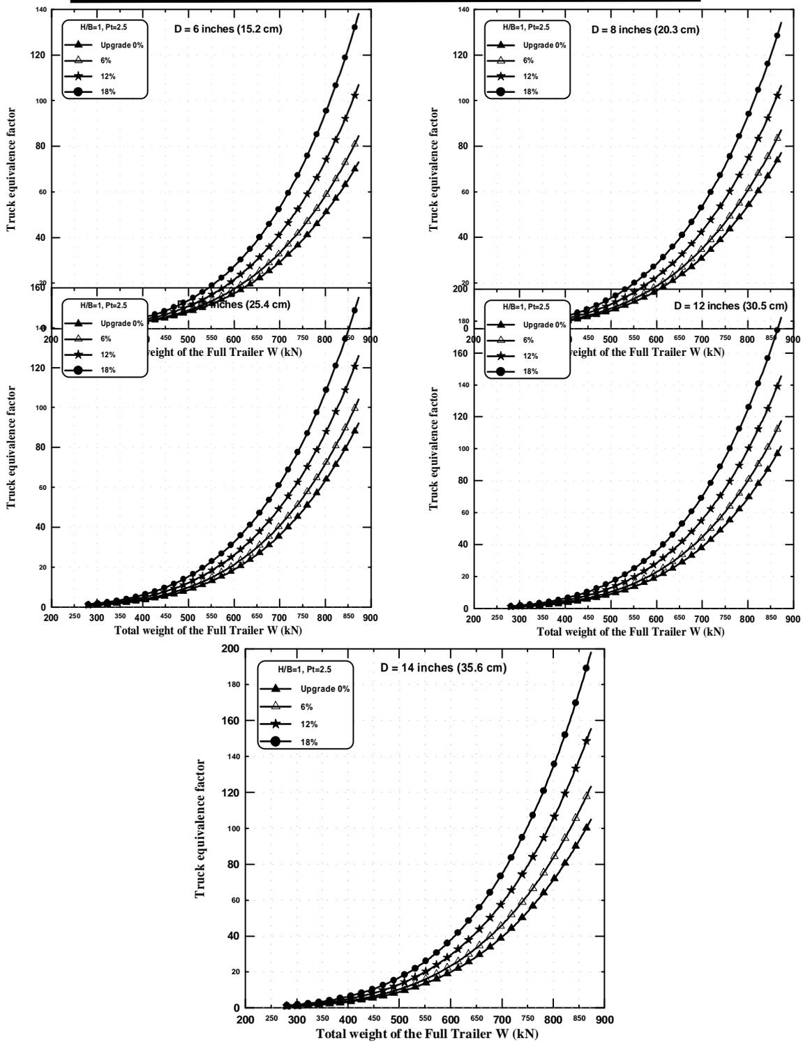
Figure (11) Equivalence factors for Full Trailers of type 1.22+2.22 on upgrades, for H/B =1.0, p<sub>t</sub>=2.5, and D=6, 8, 10, 12, and 14 inches (15.2, 20.3, 25.4, 30.5 and 35.6 cm).
