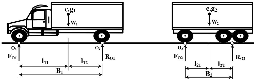
Figure (3) Forces acting on a full-trailer standing on a level road (no motion).
