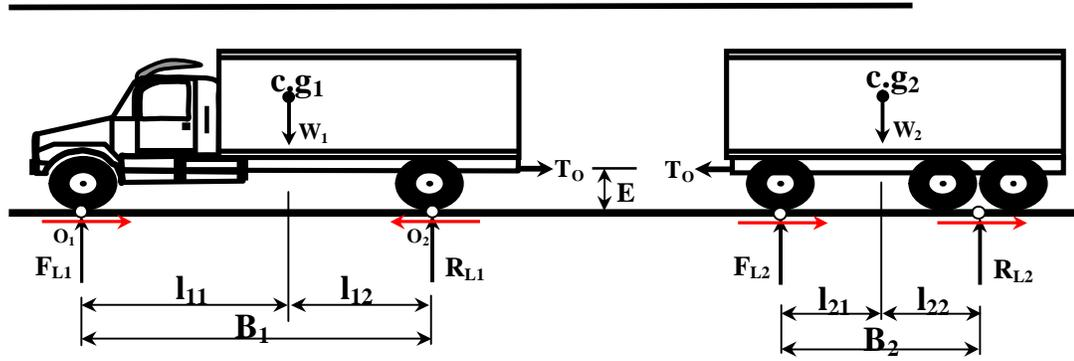
Figure (4) Forces acting on a Full-trailer on a level road moving with uniform motion.
