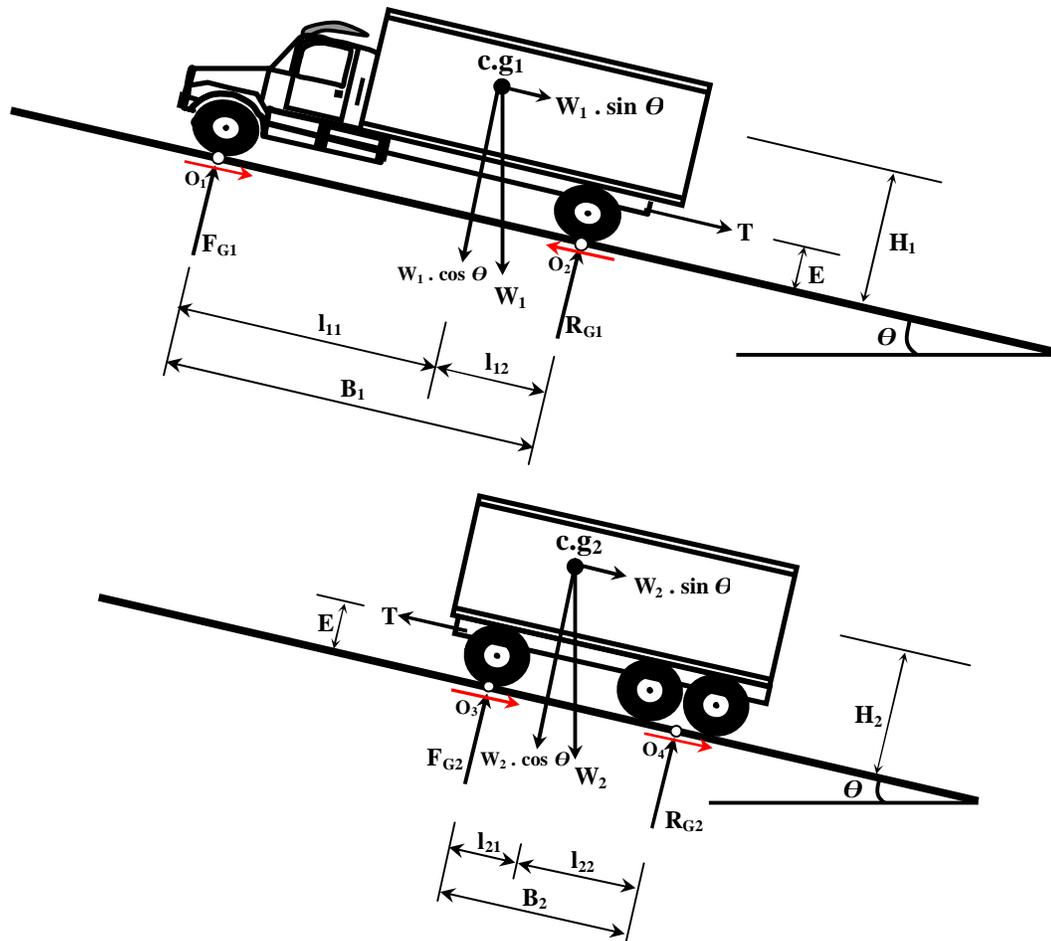
Figure (5) Forces acting on a Full-trailer moving on an upgrade with uniform motion.
