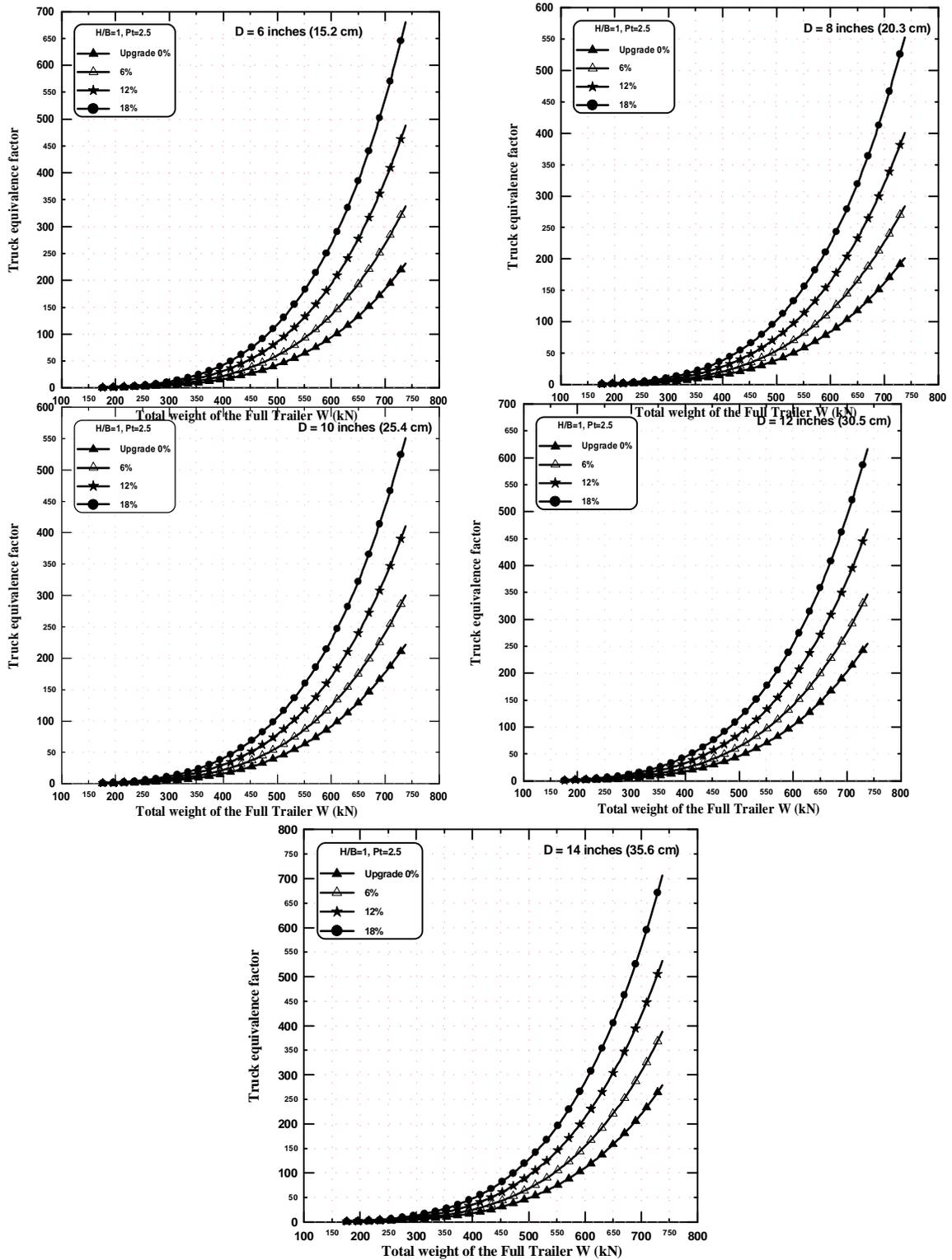
Figure (8) Equivalence factors for Full Trailers of type 1.2+2.2 on upgrades, for H/B =1.0 p<sub>t</sub>=2.5, and D=6, 8, 10, 12, and 14 inches (15.2, 20.3, 25.4, 30.5 and 35.6 cm).
