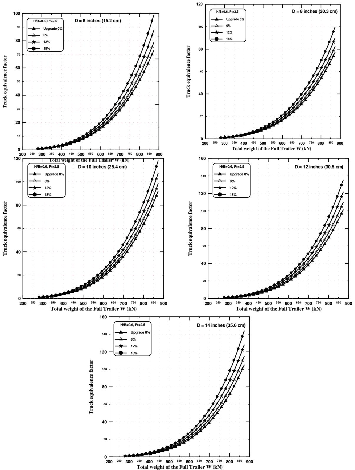
Figure (10) Equivalence factors for Full Trailers of type 1.22+2.22 on upgrades, for H/B =0.6, p=2.5, and D=6, 8, 10, 12, and 14 inches (15.2, 20.3, 25.4 , 30.5 and 35.6 cm).
