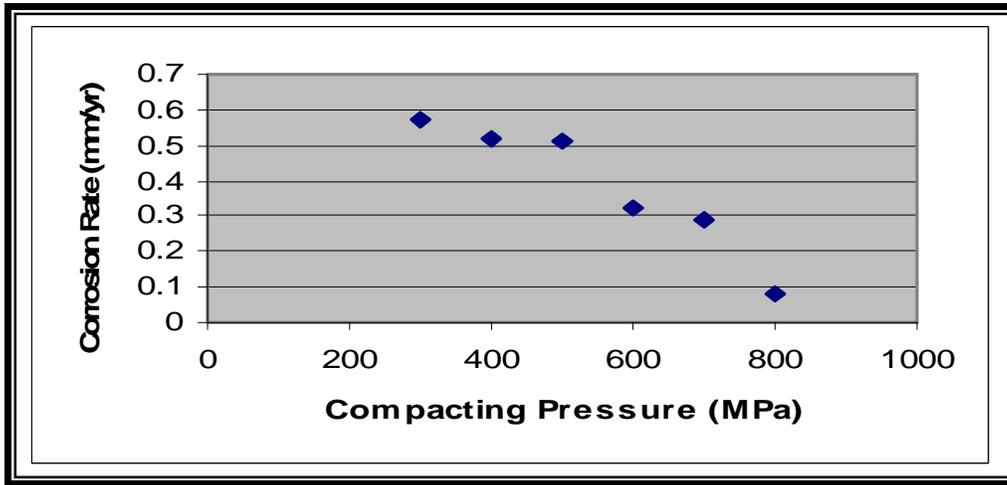
Figure (7) Corrosion rate (mm/yr) for the master sample pressed at different pressure and sintered at 950°C for 9 hrs.
