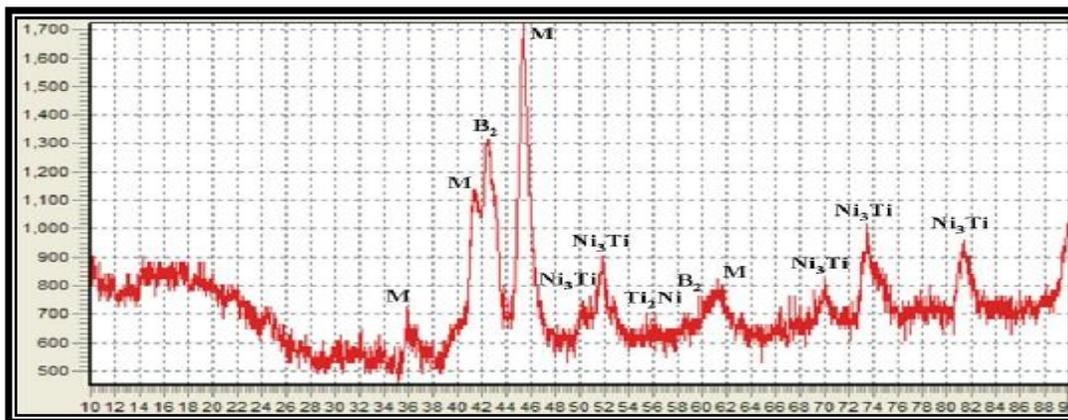
Figure (2) XRD pattern of a master sample pressed at 800MPa and sintered at 950°C for 9 hrs.
