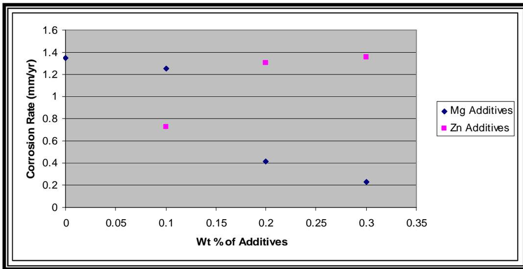
Figure (8) Corrosion rate (mm/yr) for the master with various percentages of Mg & Zn pressed at 800MPa and sintered at 950°C for 9 hrs.
