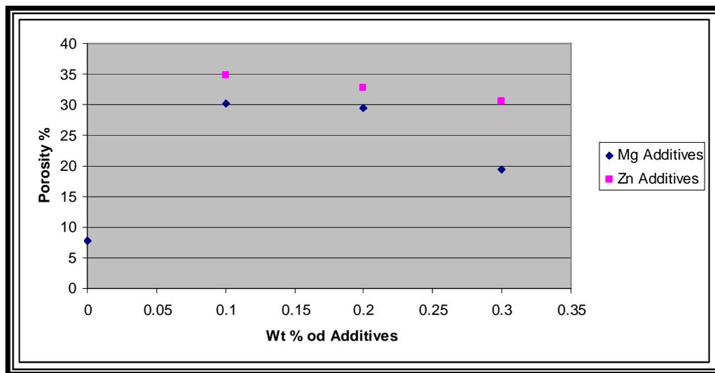
Figure (6) Porosity percentages for the master with various additives of Mg& Zn pressed at 800MPa and sintered at 950C for 9 hrs.
