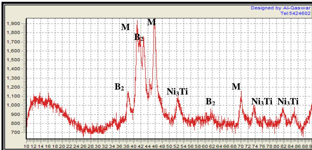
Figure (4) XRD pattern of the master with 0.3% Zn sample pressed at 800MPa and sintered at 950°C for 9 hrs.
