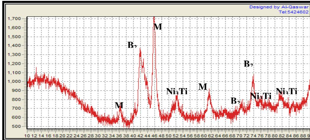
Figure (3) XRD pattern of the master with 0.3% Mg sample pressed at 800MPa and sintered at 950°C for 9 hrs
