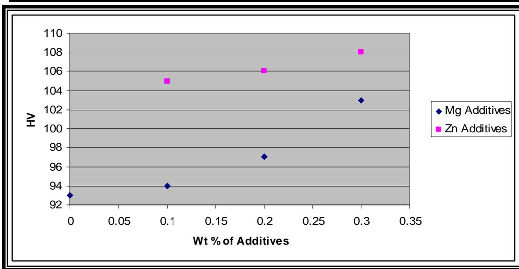
Figure (5) Hardness values for the master with various additives of Mg& Zn pressed at 800MPa and sintered at 950C for 9 hrs.
