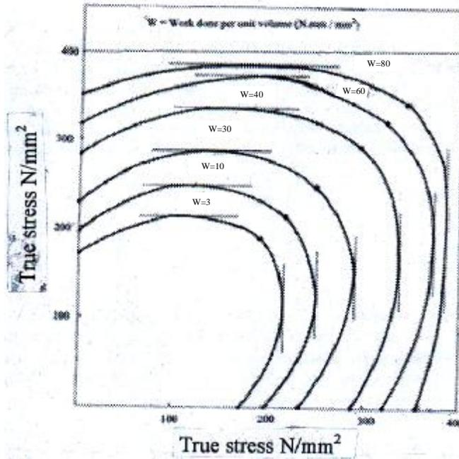
Figure (5) : Experimental yield criteria for Cu sheet drawn in open die (90°) at different work down per unit volume, W (Nmm/mm<sup>3</sup>)
