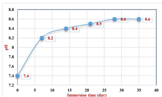
Fig. 9. Changes of pH by immersion in SBF.
