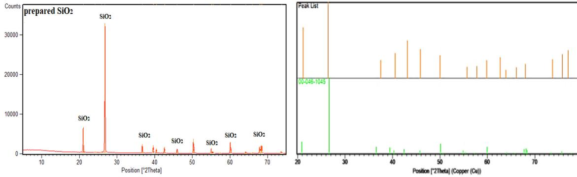
Fig. 2. XRD spectrum of prepared SiO<sub>2</sub>.
