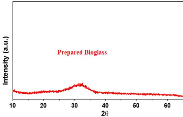
Fig. 4. XRD spectrum of prepared bioglass.
