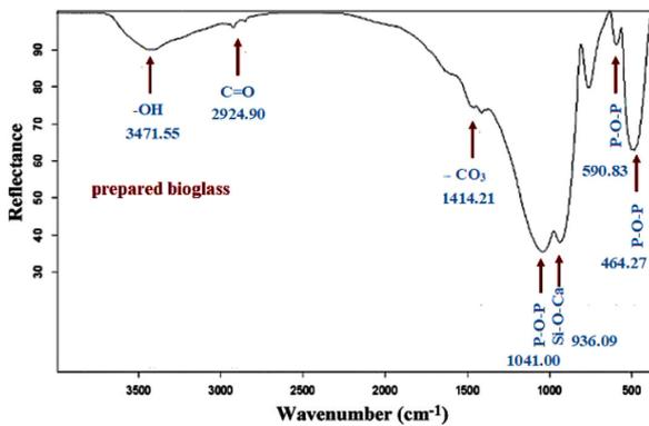
Fig. 6. FTIR spectrum of prepared bioglass.
