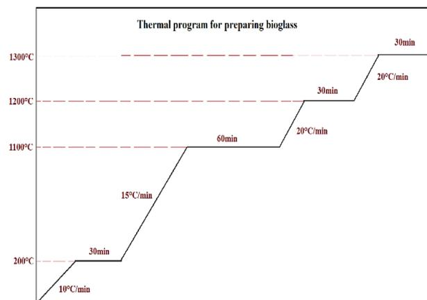
Fig. 3. Thermal program for preparing bioglass.
