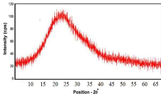
Fig. 1. XRD spectrum of glass waste.
