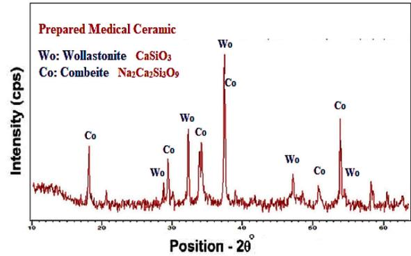
Fig. 7. XRD spectrum of prepared bioceramic.
