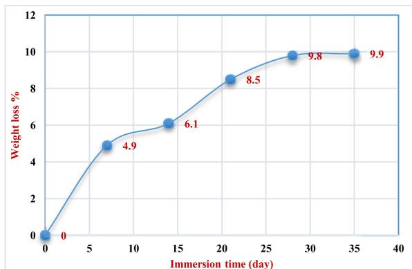
Fig. 8. Weight loss by immersion in SBF.
