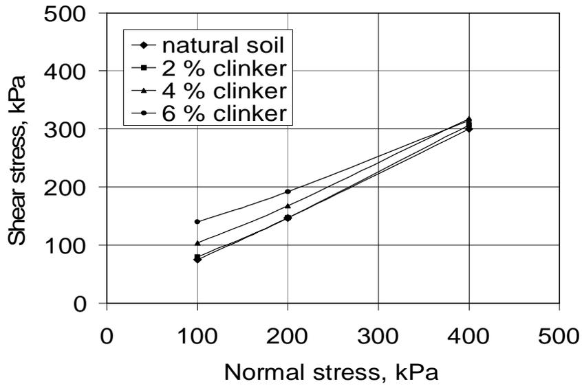
Figure (8) Results of direct shear tests.
