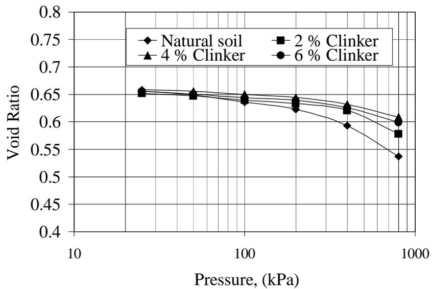
Figure (7) Applied stress vs. void ratio at unsoaking state.
