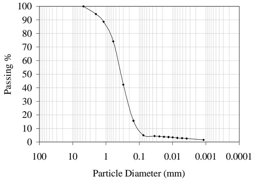
**Figure (1) – Grain size distribution for the natural soil.**
