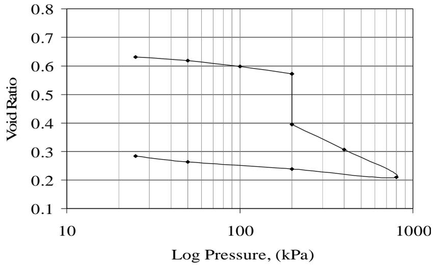
Figure (2) Results of collapse test for the natural soil.
