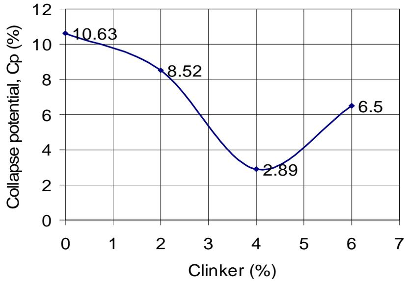
Figure (4) Effect of clinker materials on collapsibility under 200 kPa.
