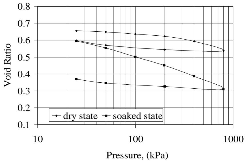
Figure (3) Results of double oedometer test for the natural soil.
