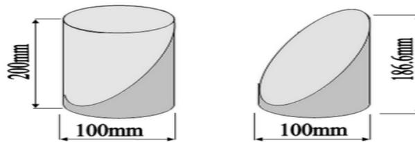
Figure (1) Substrate and composite section for slant shear bond-strength test
