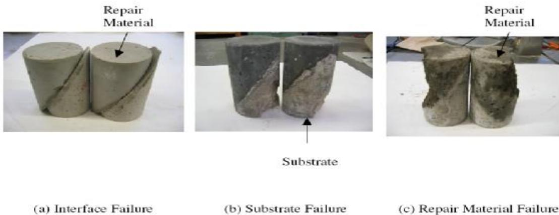
Figure (2) Failures of the composite slant sections [11].
