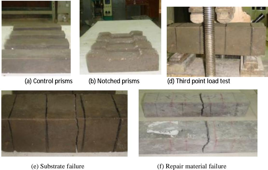
Figure (6) Compatibility test samples for composite beam of the research
