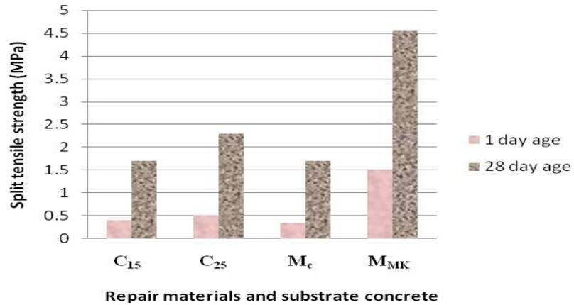
b) Split tensile strength development of repair materials with age
