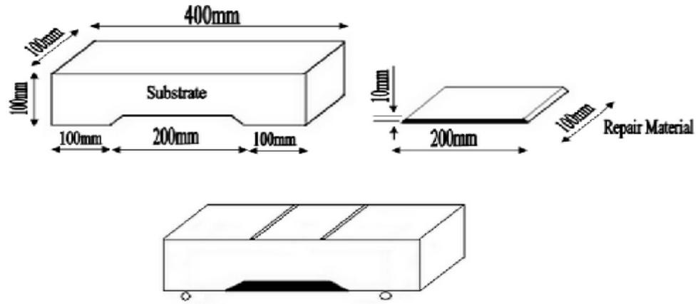
Figure (5) Third point loading composite beam
