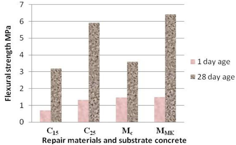
c) Flexural strength development of repair materials with age
