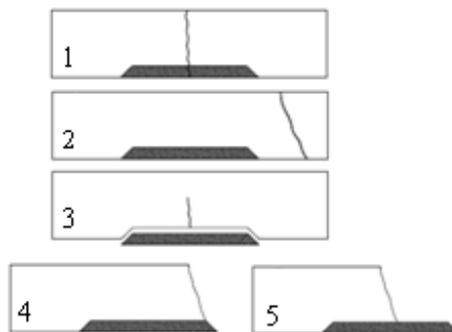
**Figure (4) Probable failures of the composite beam; 1,2 – compatible; 3, 4 and 5- incompatible [14]**
