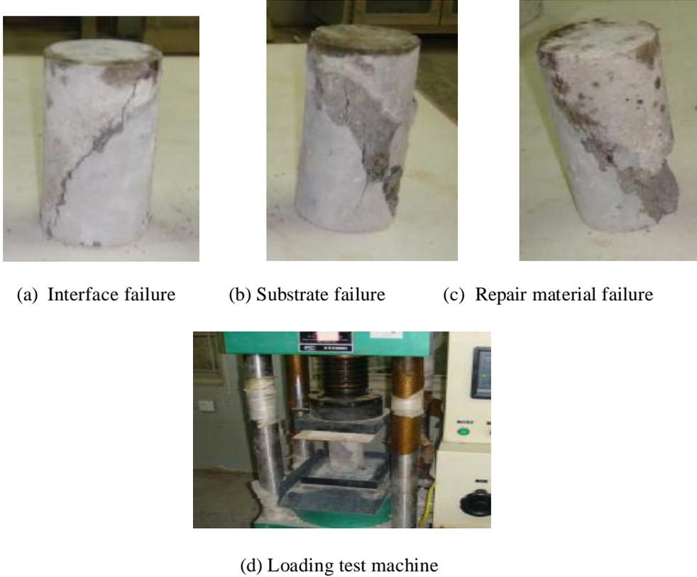
**Figure (3) Failures of the composite slant sections of the research**
