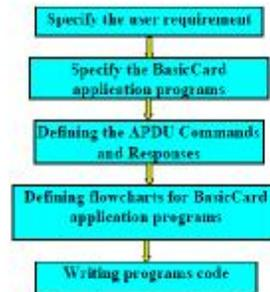
Figure (5.1): Procedure of design BasicCard application
