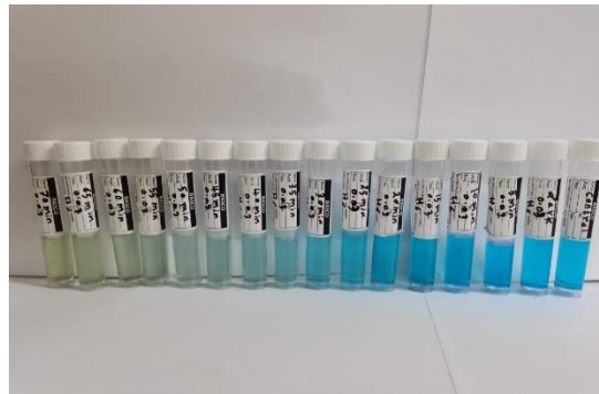
Figure 9: Illustrations showing the stages of MB dye degradation by 3 mg in 1) original dye, 2) \epsilon -Fe 2 O 3 (IONPs) in darkness, 3) after 5 minutes, 4) after 10 minutes, and 5) after 15 minutes 6) after 20 minutes, 7) by Sol-gel, and 8) after 25 minutes, till 75 minutes.
