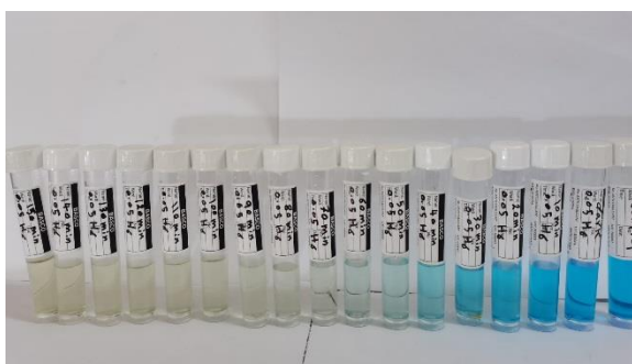
Figure 12: Illustrations of the stages involved in the 5 mg MB dye degradation: 1) using the original dye, 2) using \epsilon\text{-Fe}_2\text{O}_3 (IONPs) in the dark, 3) after 10 minutes, 4) after 20 minutes, 5) after 30 minutes, 6) after 40 minutes, 7) after 50 minutes, and so on, using the Sol-gel approach.
