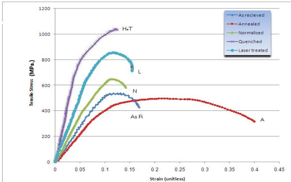
Figure (3) Stress –Strain curves for selected various heat treatments to the medium carbon steel.
