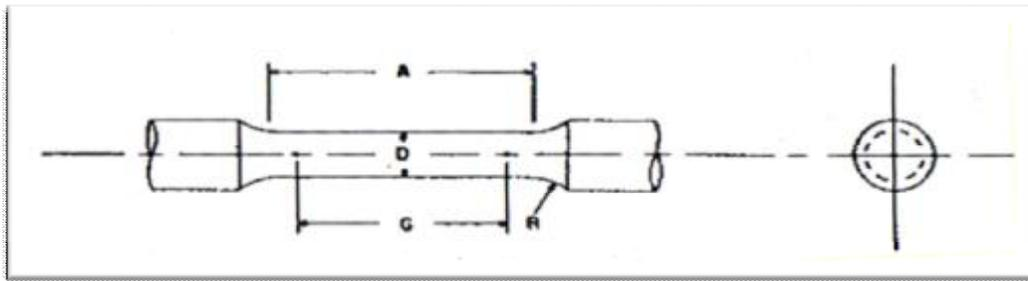
D:cross sectional diameter=4, G:gage length =16, A; length of reduced section =20, R; radius of fillet=0.08 , all dimensions in mm and the samples must obey to this relation (A=5D).
