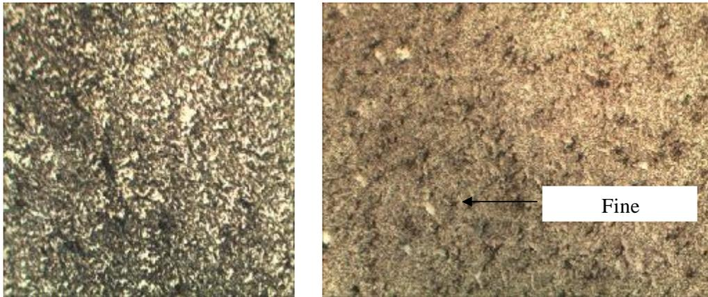
Image (5) laser surface treated core X50      Image (6) laser surface treated case X200
