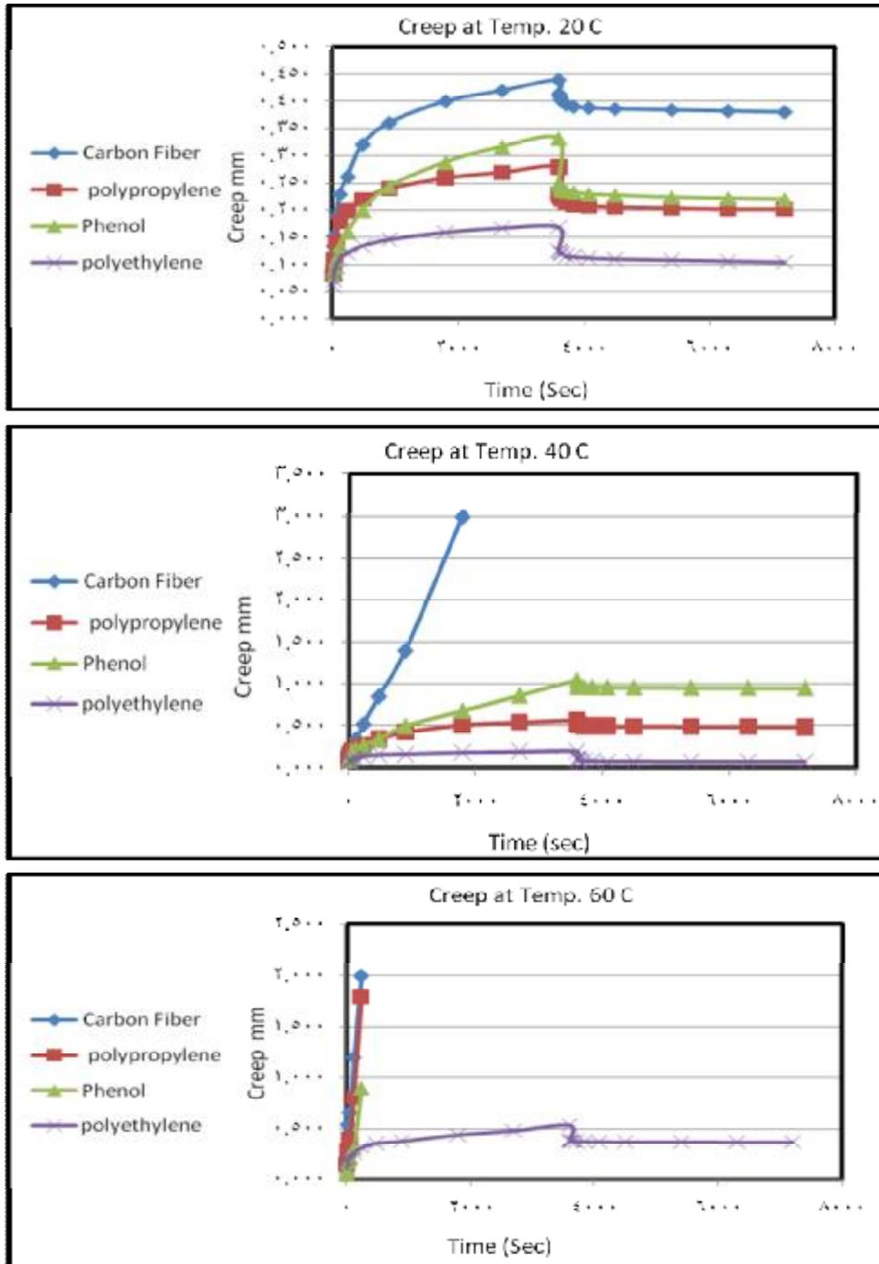
Figure (6) Creep Test at different Temperature
