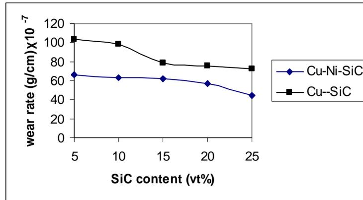
Figure (6) Variation of wear rate with Sic content for (10N) loaded
