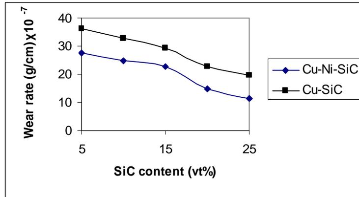
Figure (5) Variation of wear rate with Sic content for (5N) loaded
