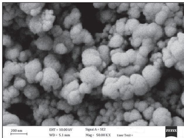
Figure 4: Field emission scanning electron microscopy image of silver nanoparticles
