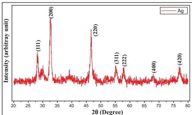
Figure 3: X-ray diffraction spectrum of synthesized silver nanoparticles
