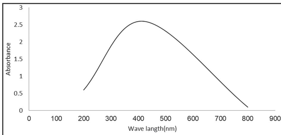
**Figure 2:** The ultraviolet–visible absorption spectrum of silver nanoparticles synthesized by *Eriobotrya japonica* seeds
