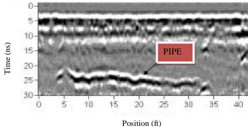
Figure (4) GPR data over a clay drainage pipe parallel to pipe direction
