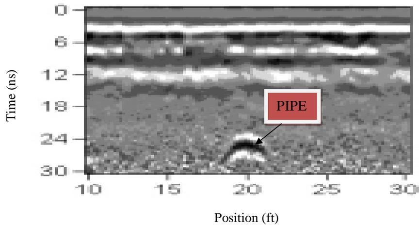
Figure (3) GPR data over clay drainage pipe perpendicular to pipe direction
