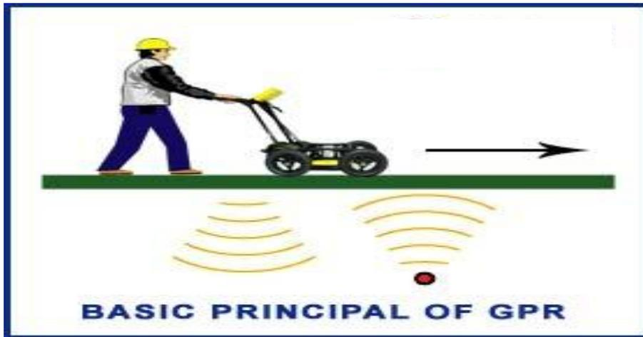
Figure (1) Basic Principle of GPR
