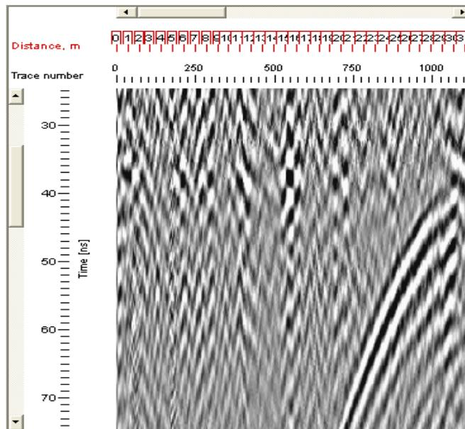
Figure (8) after (Background Removal) routine applied
