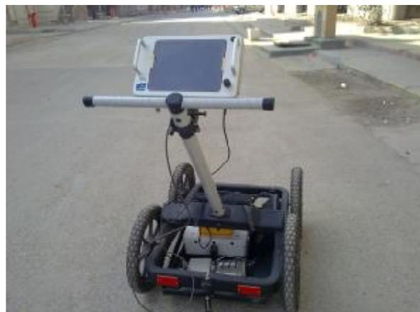
Figure (5) RAMAC/GPR System
