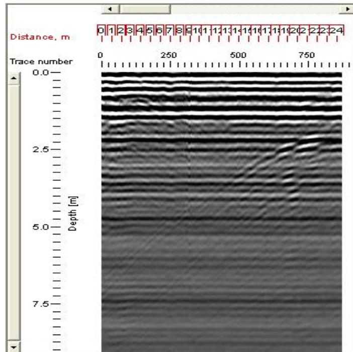
Figure (10) after (Time Adjustment) routine applied
