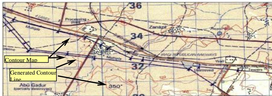
Figure (10) Zoomed part of 1<sup>st</sup> test area illustrating the generated GE contour lines (red) overlaid on topographic map (1:50,000).
