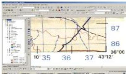
Figure (3) Geographic Coordinate system indicated in Corner of the topographical map
