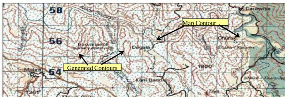
Figure (13) Zoomed part of 4<sup>th</sup> test area illustrating the generated GE contour lines (red) overlaid on topographic map (1:50,000).
