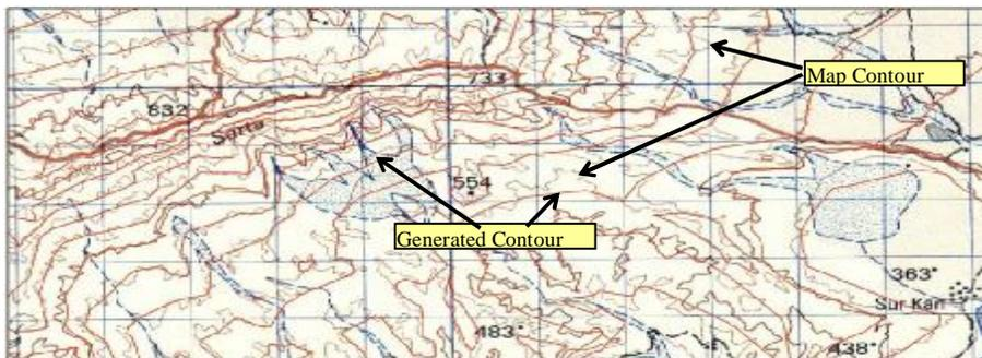
Figure (12) Zoomed part of 3<sup>rd</sup> test area illustrating the generated GE contour lines (red) overlaid on topographic map (1:50,000).
