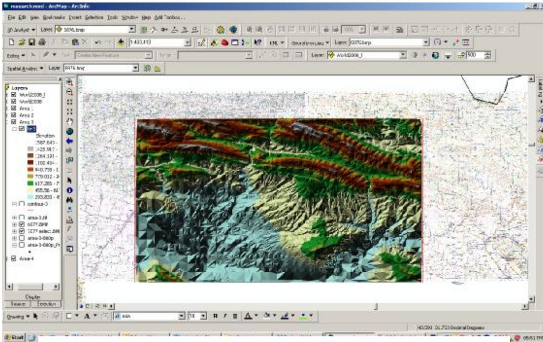
Figure (5) Triangulated Irregular Network (TIN) created for the 3<sup>rd</sup> study area.
