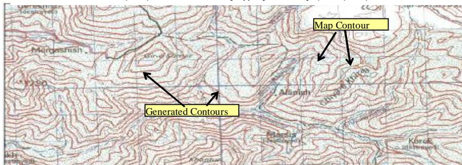
Figure (11) Zoomed part of 2<sup>nd</sup> test area illustrating the generated GE contour lines (red) overlaid on topographic map (1:50,000).
