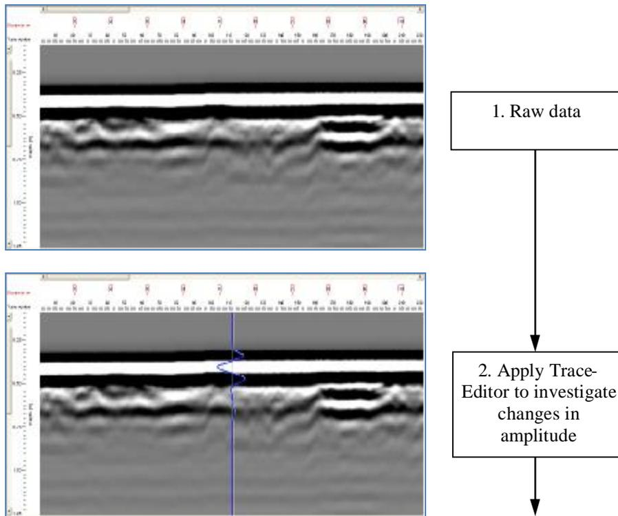
Figure (5) Typical stages in GPR data processing and presentation
