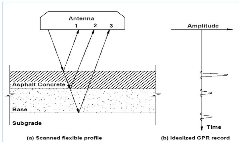
Figure (4) Methodology of determination pavement layer thickness by GPR.
