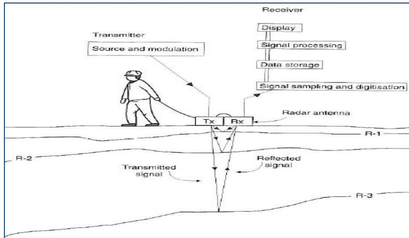
Figure (1) Sketch of basic components of a GPR system and principle of operation. [3]
