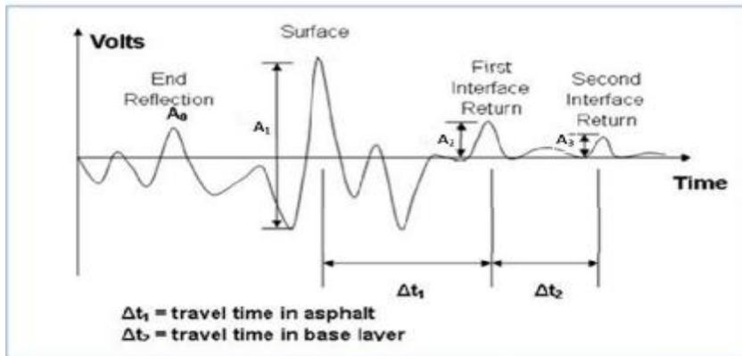
Figure (2) GPR waveform in time. [4]
