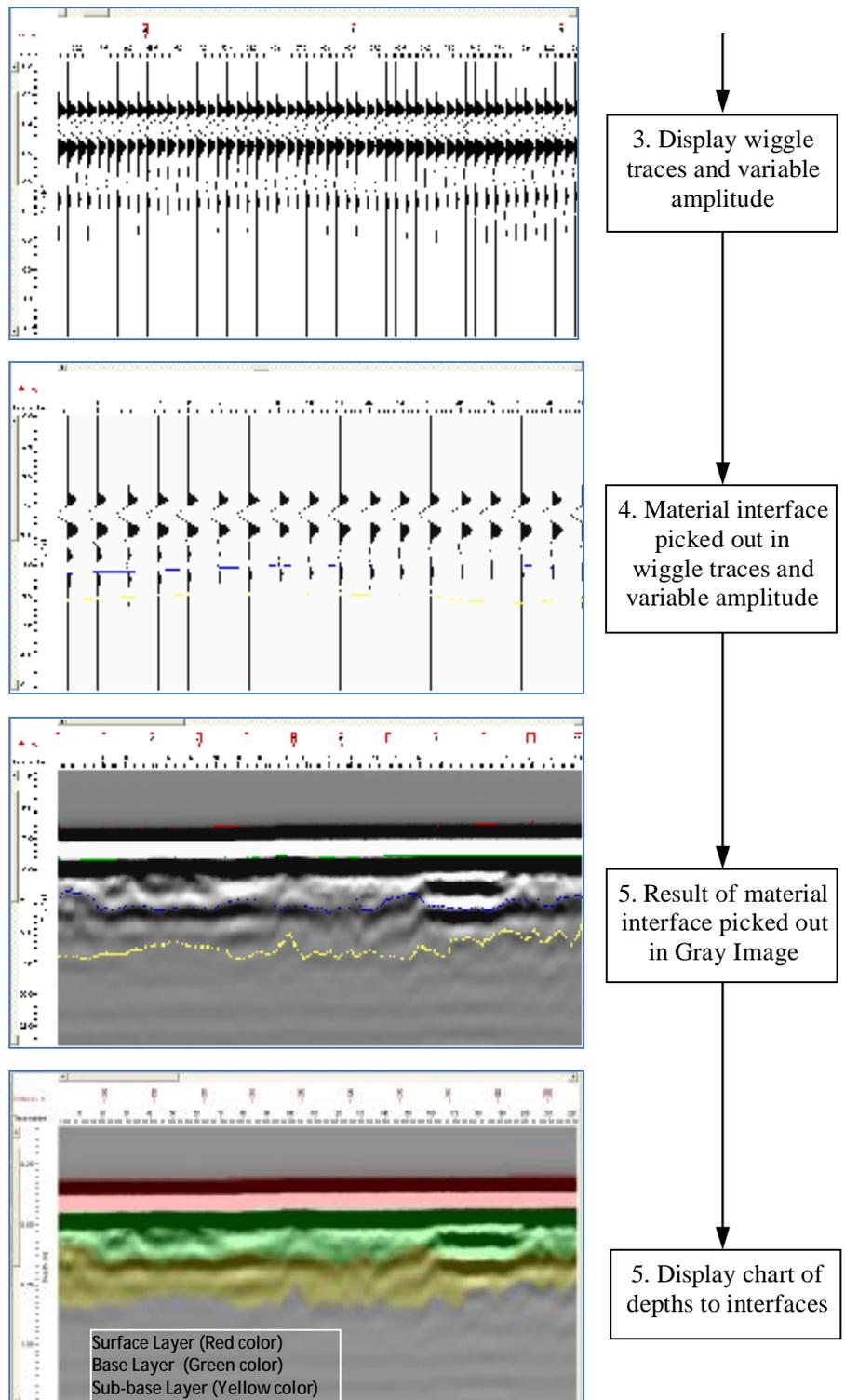
Figure (5) (continued): Typical stages in GPR data processing and
