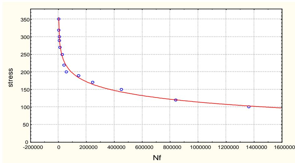
Figure (8) S-N curve of alloy 7075, notched specimens
