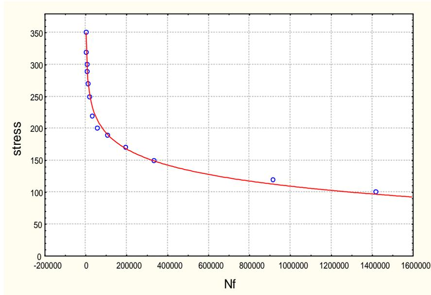
Figure (7) S-N curve of alloy 2024-T<sub>4</sub>, notched specimens
