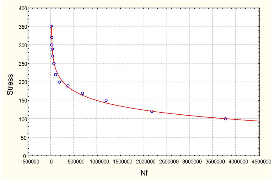
Figure (3) S-N curve of alloy (2024-T<sub>4</sub>)
