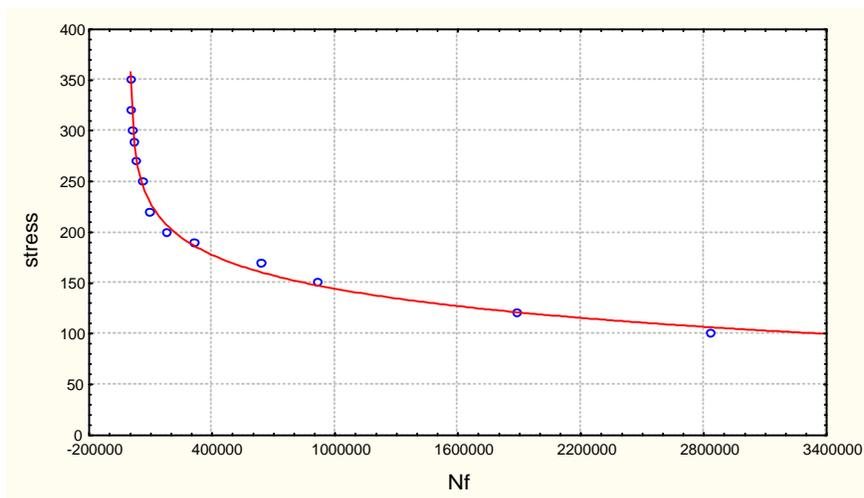
Figure (2) S-N curve of alloy 2024.
