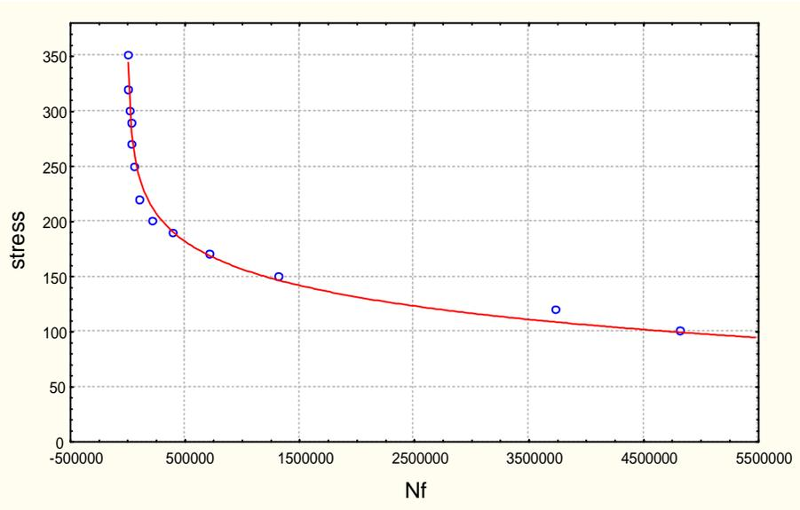
Figure (5) S-N curve of alloy 7075-T<sub>6</sub>
