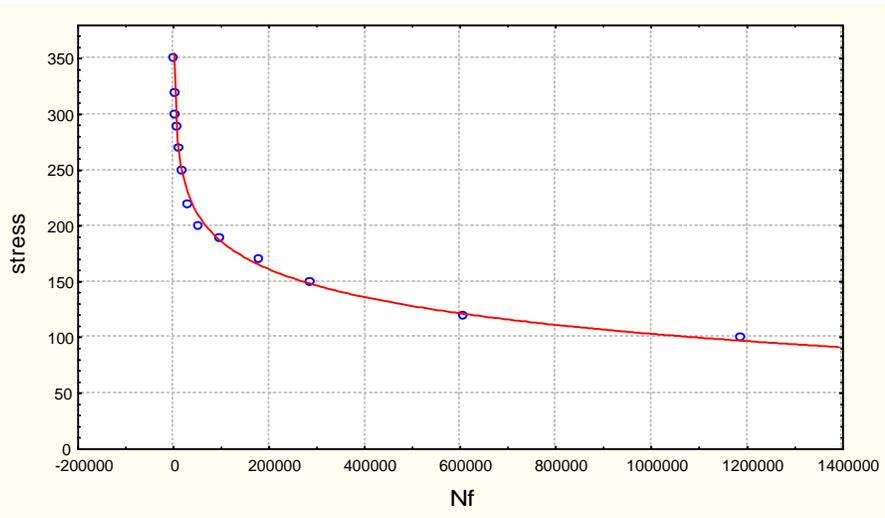
Figure (6) S-N curve of alloy 2024, notched specimens
