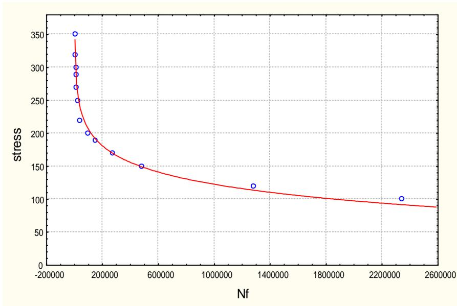
Figure (9) S-N curve of alloy 7075-T<sub>4</sub>, notched specimen
