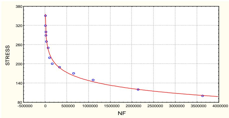
Figure (4) S-N curve of alloy 7075
