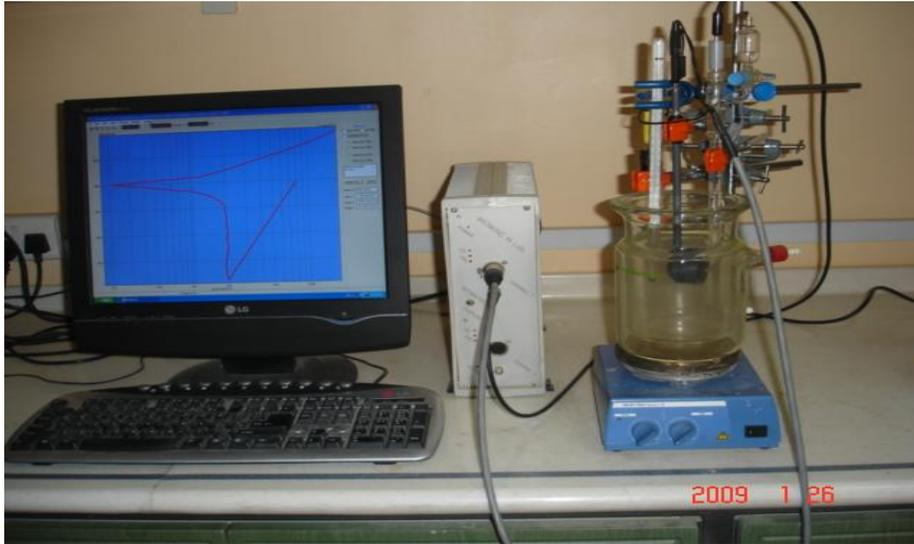
Figure ( 1 ) Potentio static equipment
