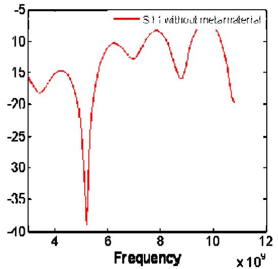
Figure.4. Simulated S<sub>11</sub> Parameter without MTM
