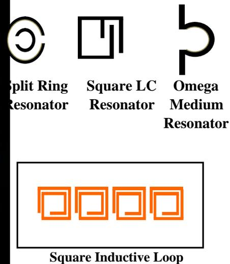
Figure3. Different Types of Resonators of MTM
