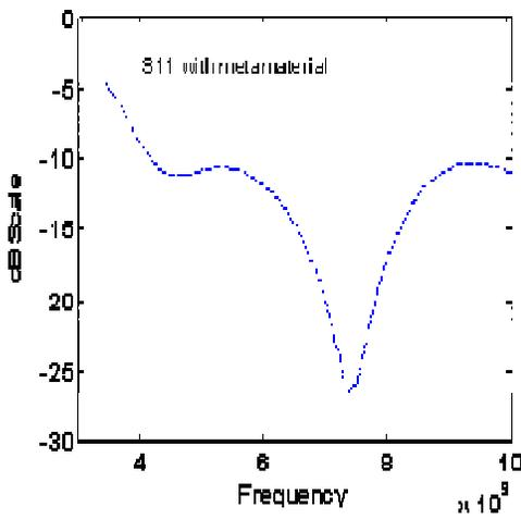
Figure.5. Simulated  $S_{11}$  Parameter of antenna with MTM
