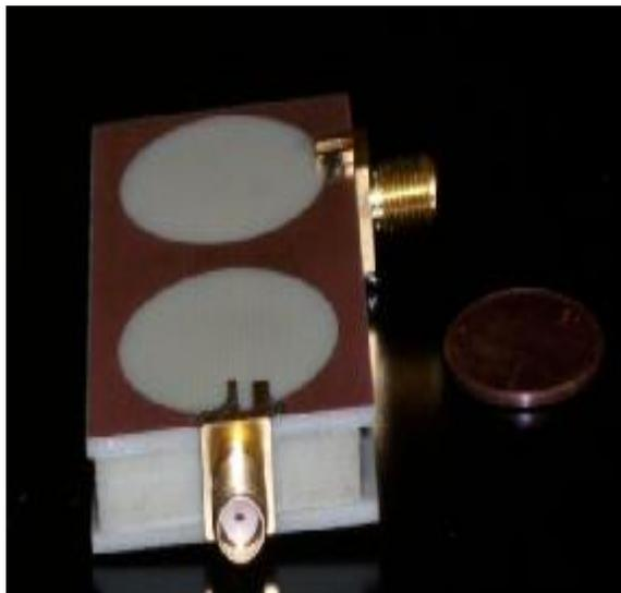
Figure.1. The structural details of the antennas prototype
