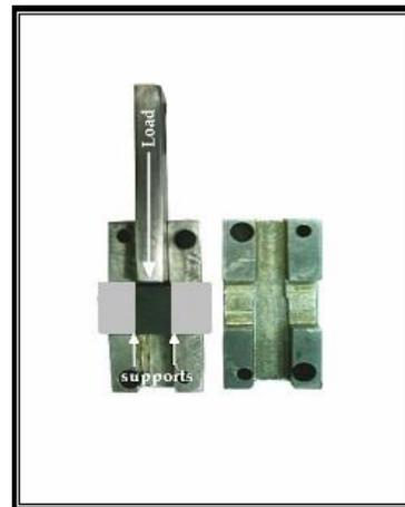
Figure (4); Punch and die used for shear test
