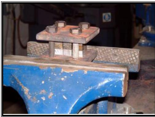
Figure (1): Fixture and assemblies for diffusion bonding double shear test specimens
