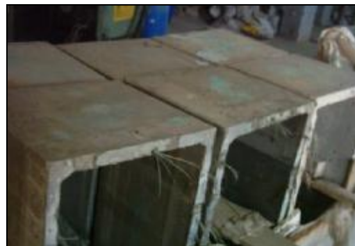
Figure (8) Specimens placed into the tank.
