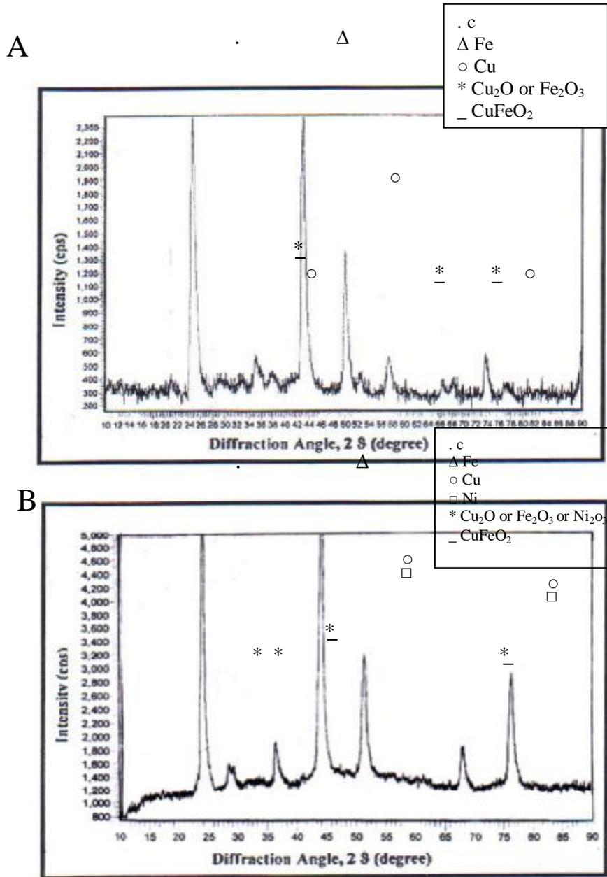
Figure (7) X- ray diffraction Analysis of alloys
