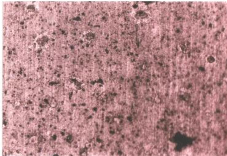
**Figure (9) Microstructure of Fe-6% Cu alloys after air -cooled.
