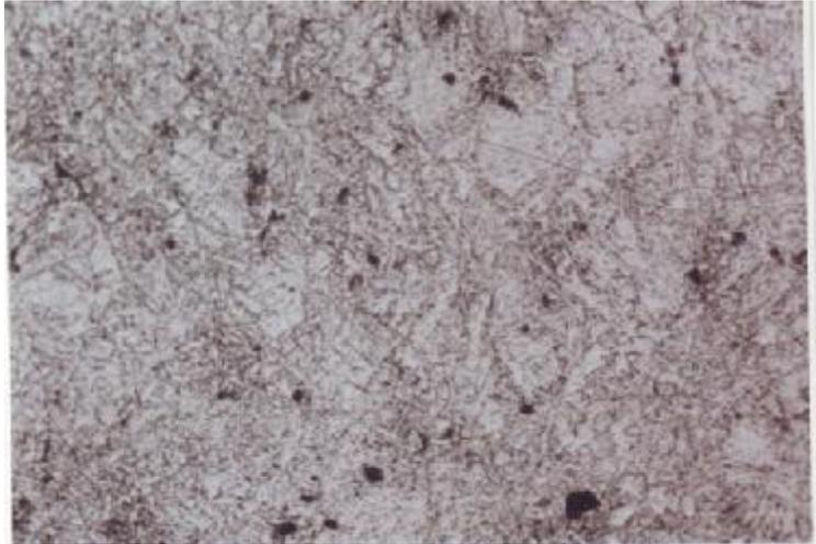
**Figure (4) Microstructure of Fe-2% Cu-1%Ni alloys after air -cooled.
