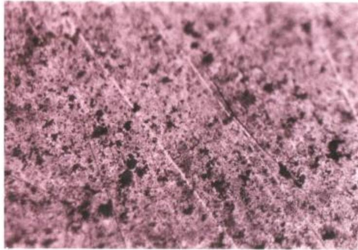
Figure (10) Microstructure of Fe-6% Cu-3%Ni alloys after air -cooled.
