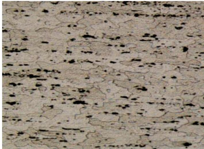
**Figure (5) Microstructure of Fe-4% Cu alloys after air -cooled.
