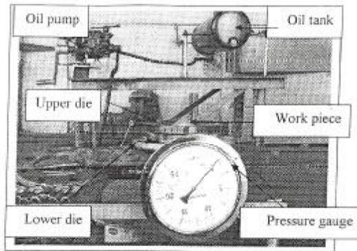
Fig 1 the equipment of hydroforming sheets metals-
