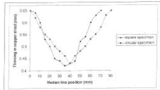
Fig 4 Thinning of sheets along the diameters lines
