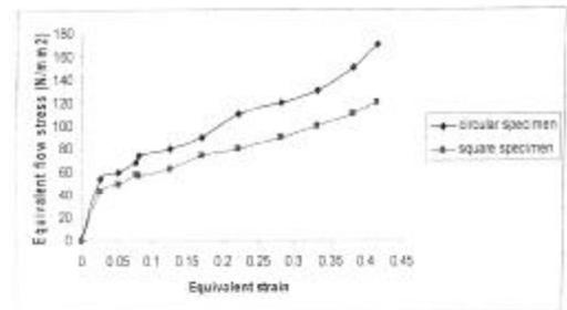
Fig 5 The relation between the equivalent stress and strain in hydroform of copper sheets
