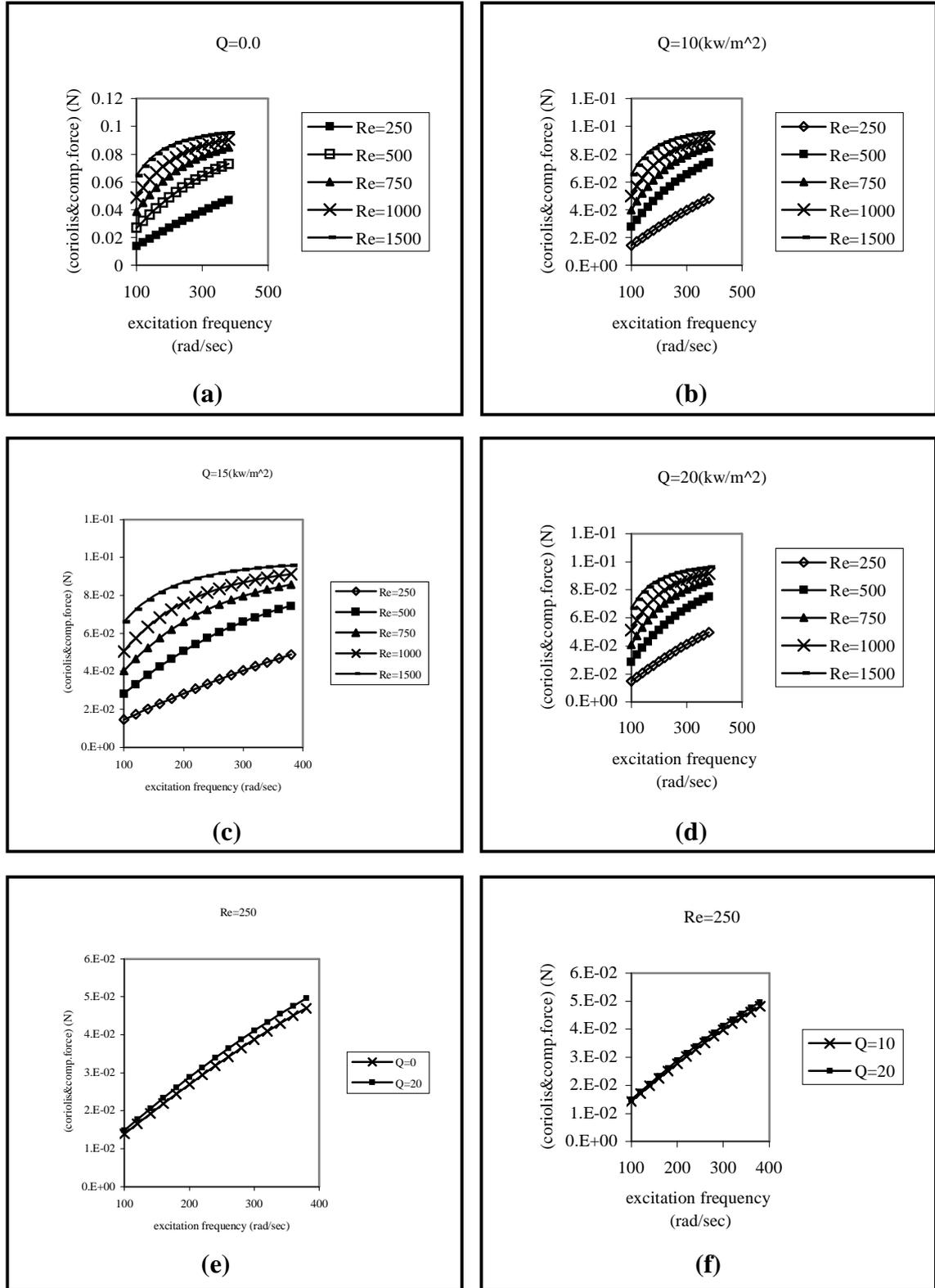
**Fig.(23) Coriolis and compressive force for simply support pipe conveying fluid due to forced vibration at mid length with various velocities and heat flux**
