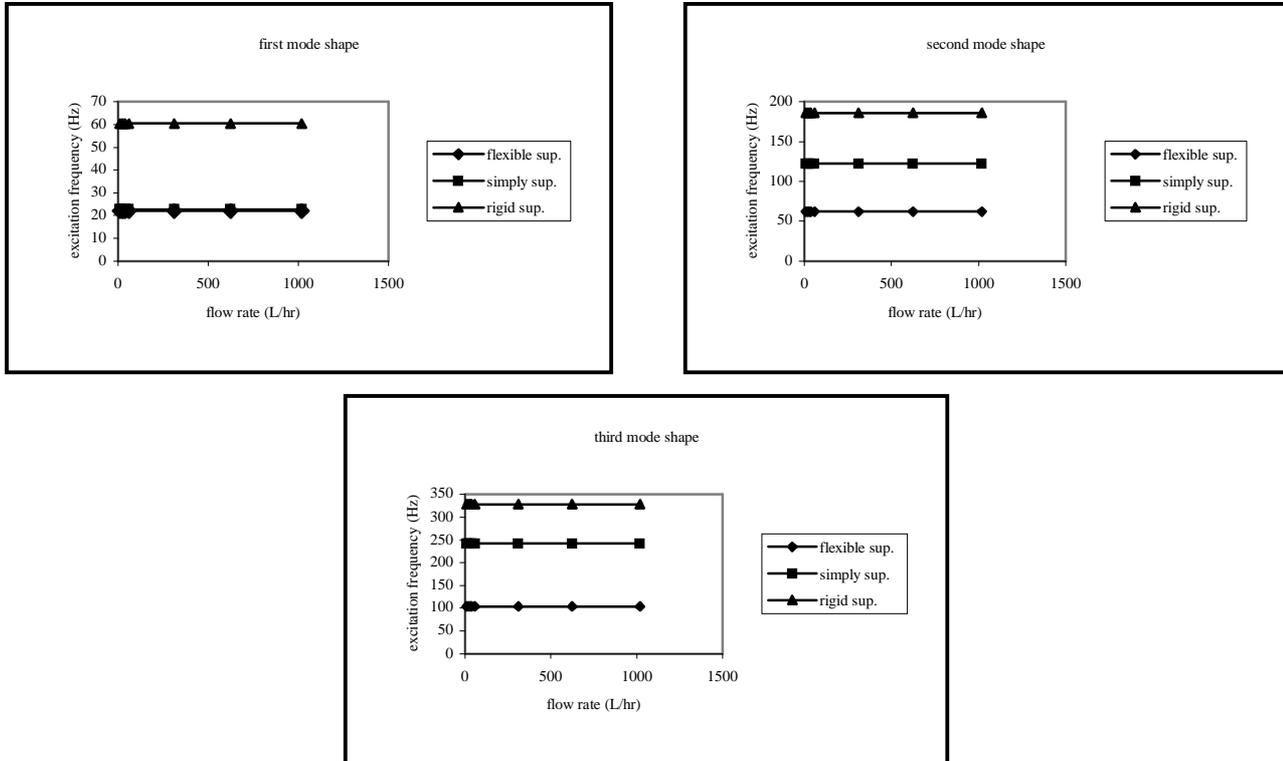
**Fig.(5) Comparison for different kinds of supports for pipe conveying fluid without heat flux**
