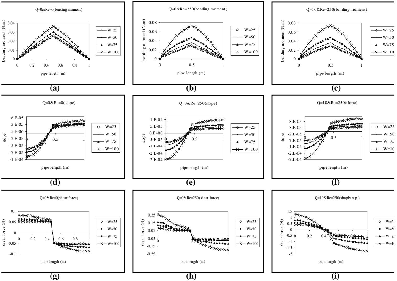
**Fig.(20) The (bending moment, slope, shear force) for simply support pipe conveying fluid with various excitation frequencies and different velocities and heat flux**
