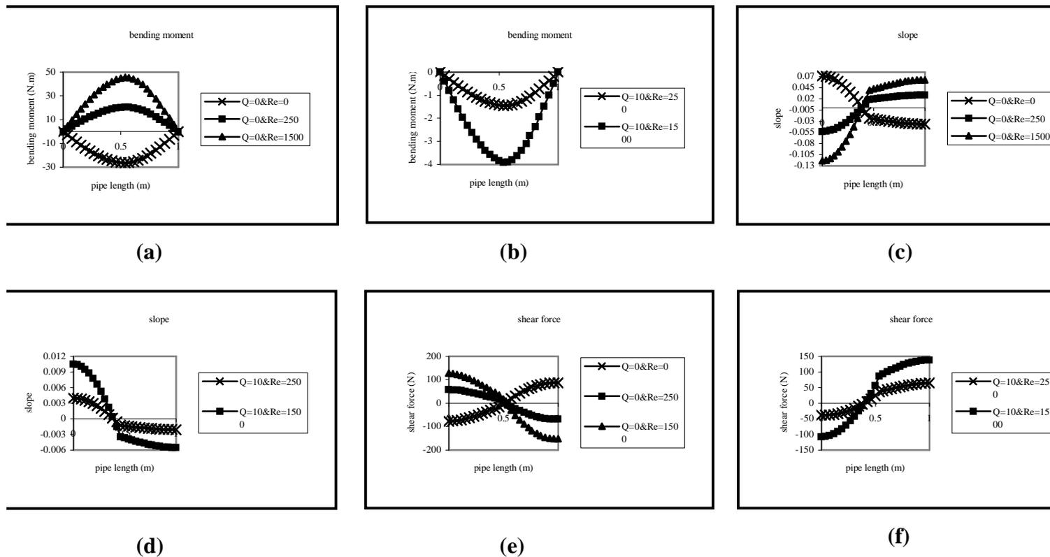
**Fig.(21) Comparison the (bending moment, slope, shear force) for simply support pipe conveying fluid at the first natural frequency and different velocities and heat flux**
