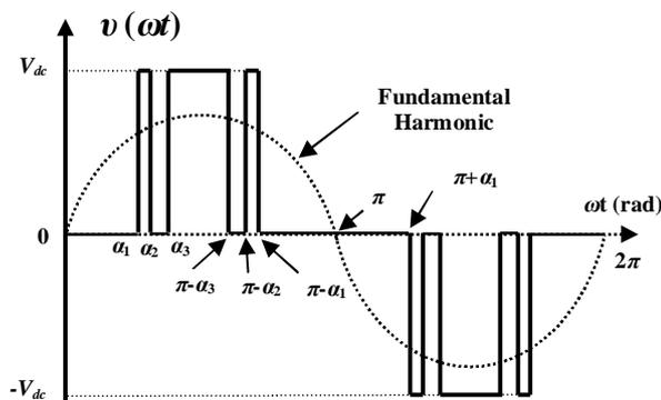
Figure (1) Unipolar PWM Switching Scheme
