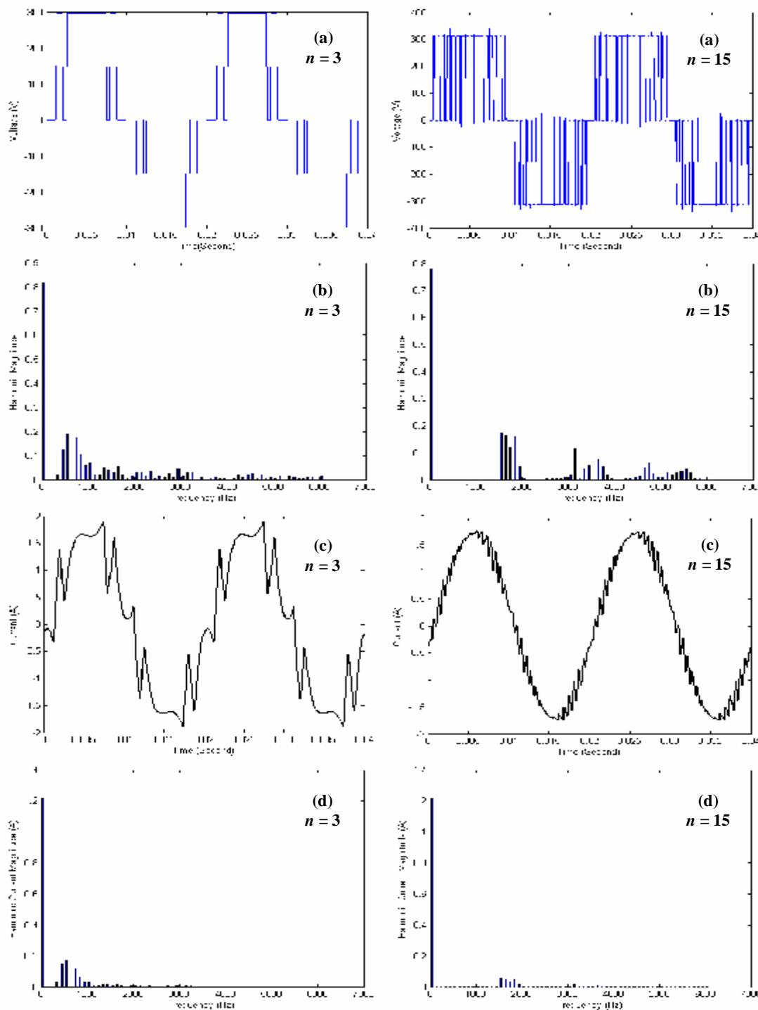
Figure (4) Shows the Instantaneous Inverter output Voltage Waveform (a), Normalized Voltage Spectra (b), Instantaneous Motor Current (c), and Motor Current Spectra (d) for 3-Level Inverter with i)  $n = 3$ ,  $m = 0.82$ , and  $THD_{min} = 43.6109$  to Eliminate the 3<sup>rd</sup> and 5<sup>th</sup> harmonics and ii)  $n = 15$ ,  $m = 0.79$ , and  $THD_{min} = 49.3008$  to Eliminate the 3<sup>rd</sup>, 5<sup>th</sup>, ..., 29<sup>th</sup> harmonics.
